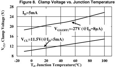
As shown in Figure 8, in the practical application of DMZ1015E/DMX1015E, with the increase of device temperature, its output voltage will also increase, and the drain-source voltage will decrease, so that the device's power consumption will also decrease. In this way, the temperature of DMZ1015E/DMX1015E will decrease. This negative feedback mechanism enables DMZ1015E/DMX1015E to reach a stable thermal equilibrium state.
