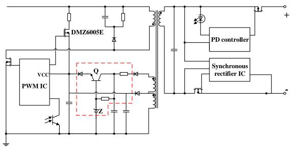
Figure 5. Normal Circuit with Transistor and Diode
