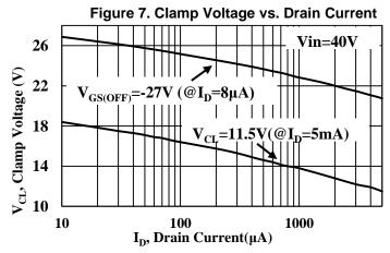
The clamping voltage will also change with the temperature. When the working temperature increases, the clamping voltage will increase; when the working temperature decreases, the clamping voltage will also decrease.
