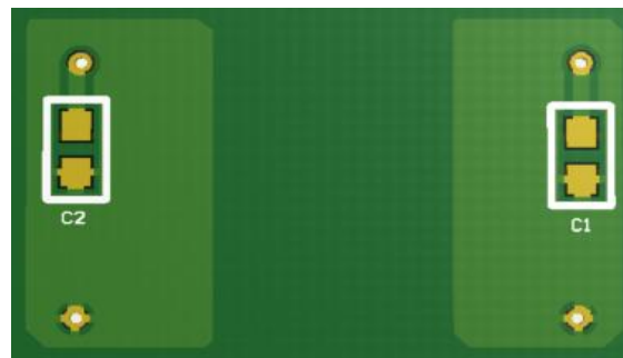
Figure 8.2 Recommended PCB Layout — Bottom Layer
