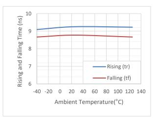
Figure 5.9 Rise and Fall time Vs Temperature
