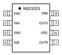
Figure. 1.1 NSD1025 Pin Configuration
