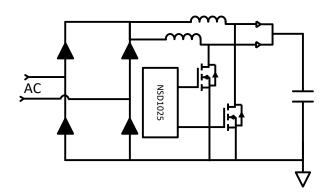
Figure 7.1 Synchronous Rectifier
