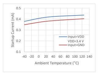
Figure 5.4 Start-up current (IDD $_{(off)}$  Vs Temperature
