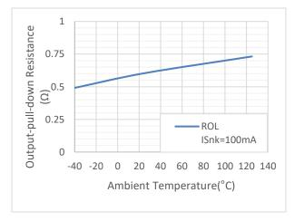
Figure 5.10 Output pull-down Resistance Vs Temperature
