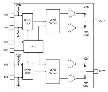
Figure 6.1 Function Block Diagram
