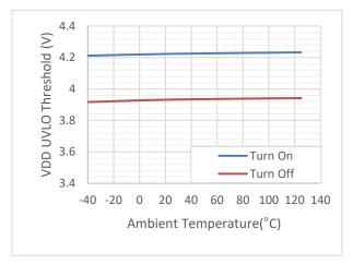
Figure 5.6 VDD UVLO Threshold Vs Temperature
