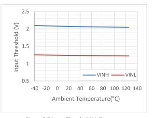
Figure 5.7 Input Threshold Vs Temperature
