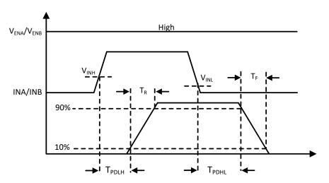
Figure 5.1 Propagation Delay, rise and fall time
