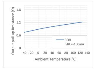
Figure 5.11 Output pull-up Resistance Vs Temperature
