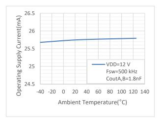
Figure 5.5 Operating supply current  $IDD_{(OP)}$  Vs Temperature
