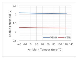
Figure 5.8 Enable threshold Vs Temperature
