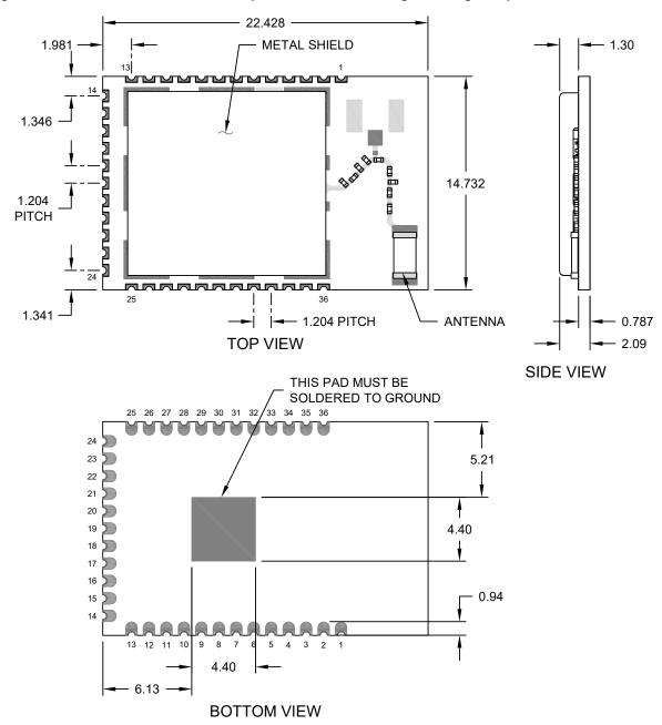
Figure 12-2. ATWINC3400-MR210CA Module Package Drawings - 3D View and Recommended Land Pattern
