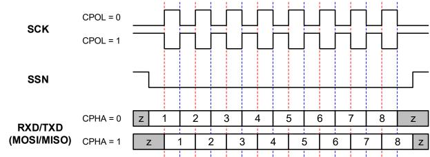
The SPI timing is provided in the following figure and table.
