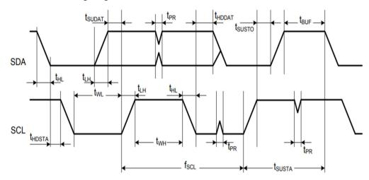
The following table provides the I<sup>2</sup>C Client timing parameters for the ATWINC3400-MR210xA module.
