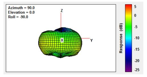
Figure 13-5. Antenna Radiation Pattern - ZX Plane
