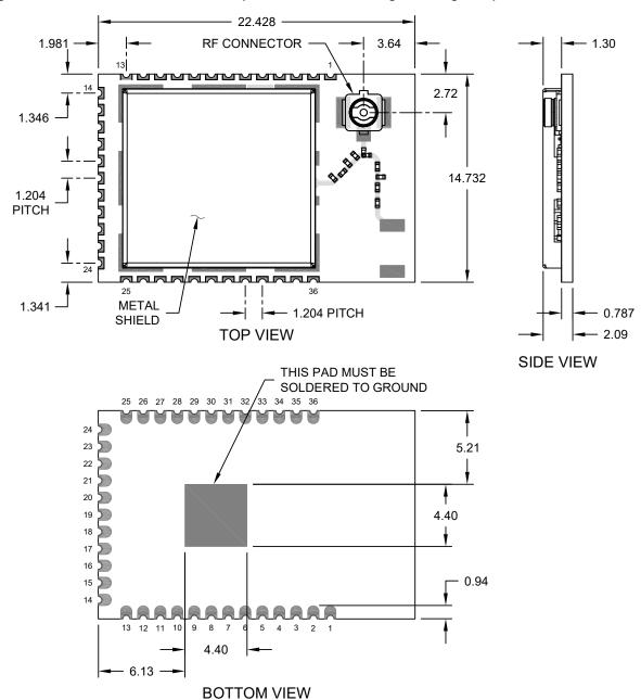
Figure 12-4. ATWINC3400-MR210UA Module Package Drawings - 3D View and Recommended Land Pattern
