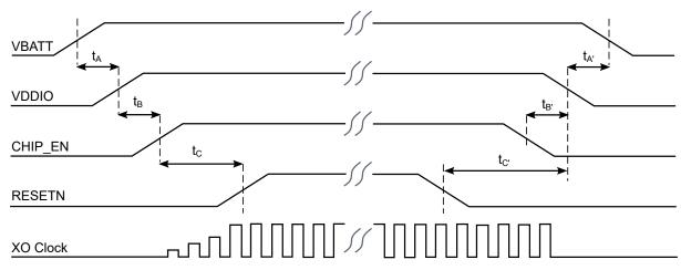
The following table provides power-up/down sequence timing parameters.
