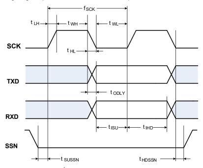
Table 10-4. SPI Client Timing Parameters(
