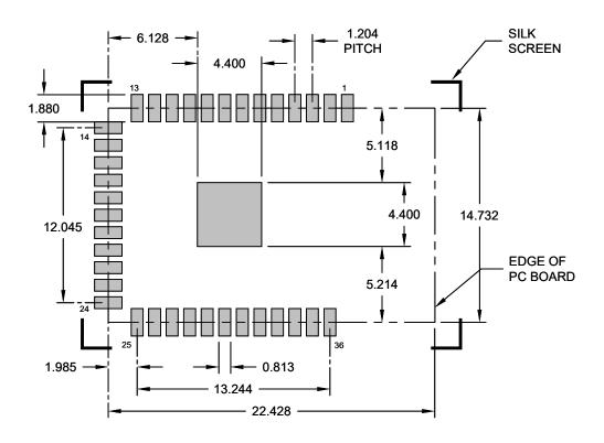
Figure 12-3. ATWINC3400-MR210UA Footprint and Module Package Drawings - Top, Bottom and Side View
