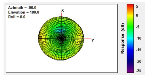
Figure 13-4. Antenna Radiation Pattern - ZY Plane
