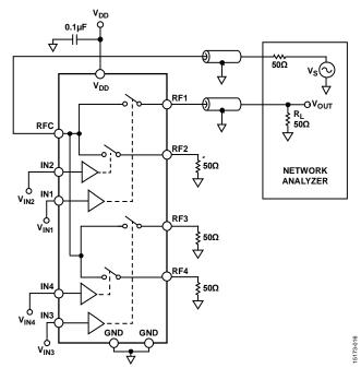
Figure 32. Isolation (All Switches Off)
