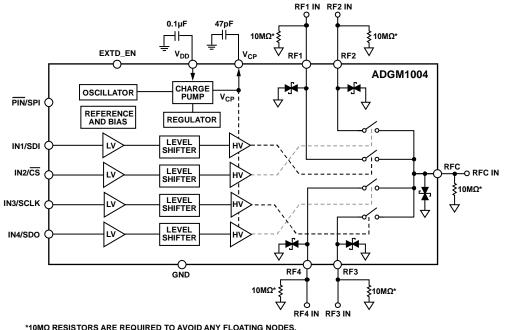
\*10MΩ RESISTORS ARE REQUIRED TO AVOID ANY FLOATING NODES. FOR MORE INFORMATION, REFER TO THE CRITICAL OPERATIONAL REQUIREMENTS SECTION NOTES 1. LV = LOW VOLTAGE. HV = HIGH VOLTAGE.
