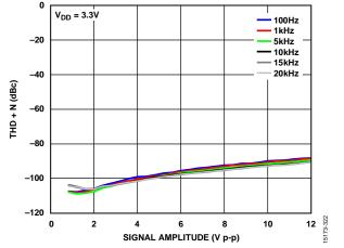
Figure 23. THD + N vs. Signal Amplitude ( $V_{DD} = 3.3 V$ ,  $R_{LOAD} = 300 \Omega$ ,  $T_A = 25 °C$ , Signal Source Impedance =  $20 \Omega$ )
