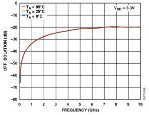
Figure 18. Off Isolation vs. Frequency over Temperature, All Channels Off ( $V_{DD} = 3.3 V$ , RF1 to RFC)
