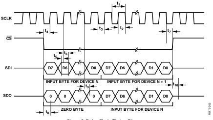
Figure 3. Daisy-Chain Timing Diagram
