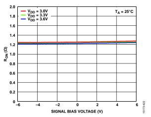
Figure 11. R<sub>ON</sub> vs. Signal Bias Voltage over Supply Voltages (Measured 5 sec Post Switch Turn On Time, RF1 to RFC on)
