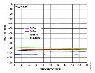
Figure 24. THD + N vs. Frequency ( $V_{DD}$  = 3.3 V,  $R_{LOAD}$  = 300  $\Omega$ ,  $T_A$  = 25°C, Signal Source Impedance = 20  $\Omega$
