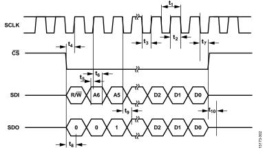
Figure 2. Addressable Mode Timing Diagram
