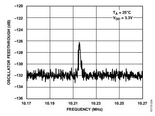
Figure 29. Oscillator Feedthrough vs. Frequency, Zoomed in at 10.2 MHz  $(V_{\text{DD}} = 3.3 \text{ V})$
