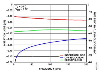
Figure 16. Insertion Loss and Off Isolation/Return Loss vs. Frequency  $(V_{DD} = 3.3 V, RF1 \text{ to } RFC)$
