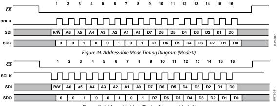
Figure 45. Addressable Mode Timing Diagram (Mode 3)
