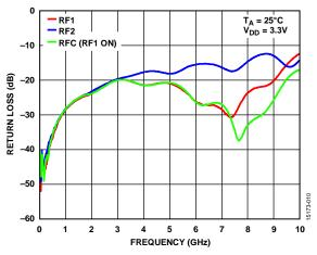
Figure 20. Return Loss vs. Frequency ( $V_{DD} = 3.3 V$ )
