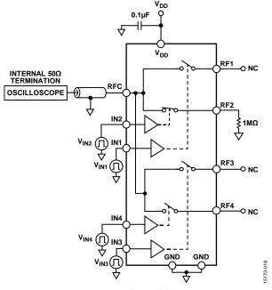
Figure 35. Video Feedthrough
