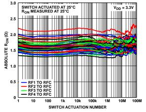
Figure 6. Absolute  $R_{ON}$  vs. Switch Actuation Number, Switch Actuated at 25°C and  $R_{ON}$  Measured at 25°C
