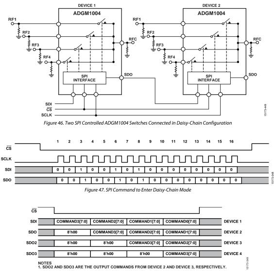
Figure 48. Example of SPI Frame with Three ADGM1004 Switches Connected in Daisy-Chain Mode
