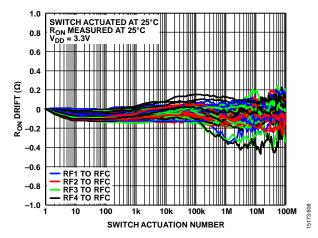
Figure 7. Ron Drift vs. Switch Actuation Number, Normalized at Zero, Switch Actuated at  $25^{\circ}$ C and Ron Measured at  $25^{\circ}$ C
