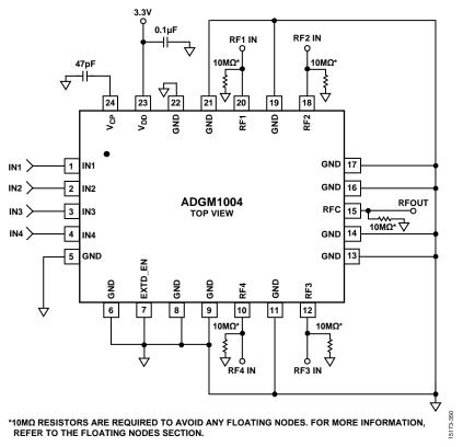
Figure 49. Typical Operating Circuit
