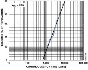
Figure 62. Cumulative On Switch Lifetime at 50°C,  $V_{DD} = 3.3 V$ , Sample Size 31 Parts
