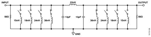
Figure 52. Reconfigurable Band-Pass Filter Achieved Using Two ADGM1004 MEMS Switches
