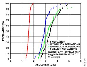
Figure 54. Population Percentage vs. Absolute  $R_{ON_r}$  Switch Actuated at 85°C and  $R_{ON}$  measured at 25°C
