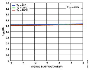
Figure 12. Row vs. Signal Bias Voltage over Temperature (Measured 5 sec Post Switch Turn On Time, RF1 to RFC on)
