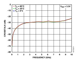
Figure 22. Crosstalk vs. Frequency over Temperature ( $V_{DD} = 3.3 V$ , RF2 to RF1)
