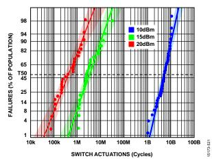
Figure 13. Hot Switching Probability Distribution on Log Normal with 95% Confidence Interval (CI) (RF Power = CW, Terminated into 50  $\Omega$ ,  $T_A = 25^{\circ}$ C,  $V_{DD} = 3.3 V$ )
