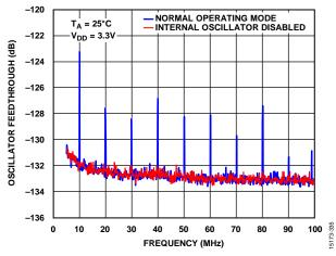
Figure 30. Oscillator Feedthrough vs. Frequency, Wide Bandwidth  $(V_{DD} = 3.3 V)$
