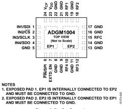
Figure 5. Pin Configuration
