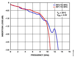
Figure 14. Insertion Loss vs. Frequency, Linear Scale ( $V_{DD} = 3.3 V$ )
