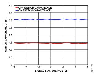
Figure 26. Switch Capacitance vs. Signal Bias Voltage
