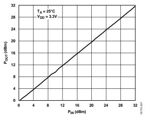
Figure 27. Output Power ( $P_{OUT}$ ) vs. Input Power ( $P_{IN}$ ) ( $V_{DD}$  = 3.3 V, Signal Frequency = 4 GHz)
