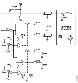
Figure 31. Insertion Loss and Return Loss
