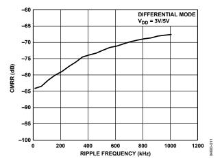
Figure 15. CMRR vs. Common-Mode Ripple Frequency
