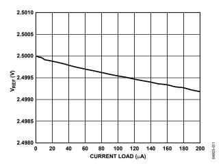
Figure 12. V<sub>REF</sub> vs. Reference Output Current Drive
