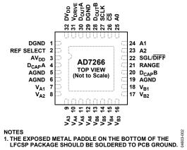
Figure 2. Pin Configuration (CP-32-7)
