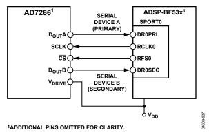
Figure 44. Interfacing the AD7266 to the ADSP-BF53x
