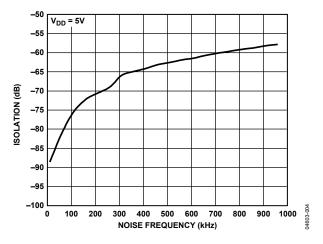
Figure 5. Channel-to-Channel Isolation
