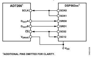
Figure 46. Interfacing the AD7266 to the DSP563xx
