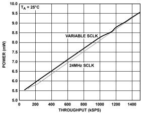
Figure 39. Power vs. Throughput in Normal Mode with  $V_{\rm DD} = 3 \ V$
