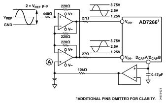
Figure 26. Dual Op Amp Circuit to Convert a Single-Ended Unipolar Signal into a Differential Sianal
