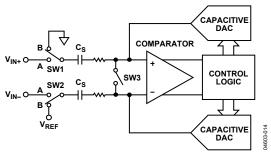
Figure 17. ADC Conversion Phase
