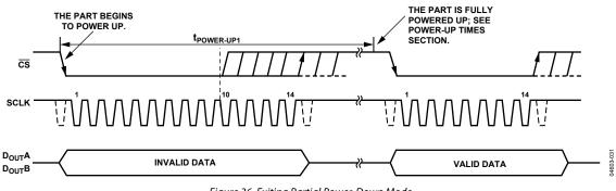
Figure 36. Exiting Partial Power-Down Mode
