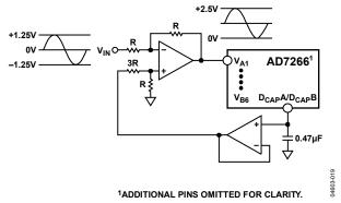
Figure 22. Single-Ended Mode Connection Diagram
