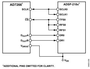
Figure 43. Interfacing the AD7266 to the ADSP-218x
