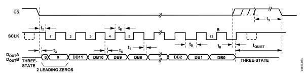
Figure 41. Serial Interface Timing Diagram
