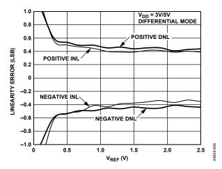
Figure 10. Linearity Error vs. V<sub>REF</sub>
