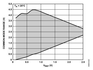
Figure 25. Input Common-Mode Range vs.  $V_{REF}$  (2 ×  $V_{REF}$  Range,  $V_{DD}$  = 5 V)
