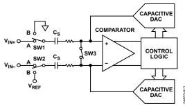
Figure 16. ADC Acquisition Phase
