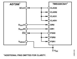
Figure 45. Interfacing the AD7266 to the TMS320C541
