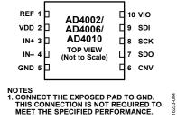
Figure 3. 10-Lead MSOP Pin Configuration
