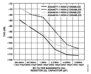
Figure 46. THD vs. RC Bandwidths for Various Precision ADC Drivers,  $f_{\rm IN}=1$  kHz (Turbo Mode On, High-Z Enabled/Disabled), VDD = 1.8 V, VIO = 3.3 V,  $V_{\rm REF}=5$  V,  $T_{\rm A}=25$ °C
