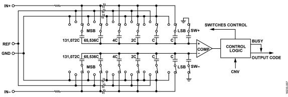
Figure 37. ADC Simplified Schematic
