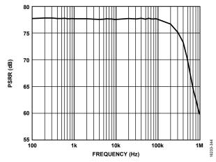
Figure 32. PSRR vs. Frequency, VDD = 1.8 V, VIO = 3.3 V,  $V_{REF} = 5 \text{ V}$ ,  $T_A = 25 ^{\circ}\text{C}$
