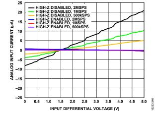
Figure 28. Analog Input Current vs. Input Differential Voltage
