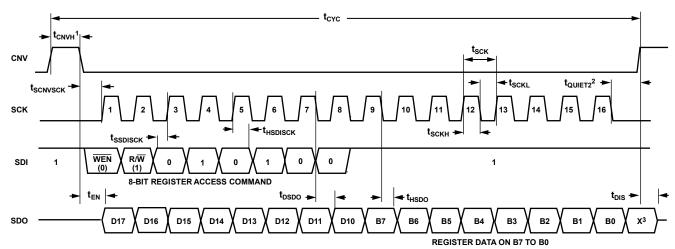
$^1\text{THE}$  CNV HIGH TIME MUST FOLLOW THE  $t_{\text{CONV}}$  SPECIFICATION TO GENERATE A VALID CONVERSION RESULT  $^2\text{THE}$  SCK FALLING EDGE TO CNV RISING EDGE DELAY MUST FOLLOW THE  $t_{\text{QUIET2}}$  SPECIFICATION TO ENSURE SPECIFIED PERFORMANCE  $^3\text{X}$  MEANS DON'T CARE
