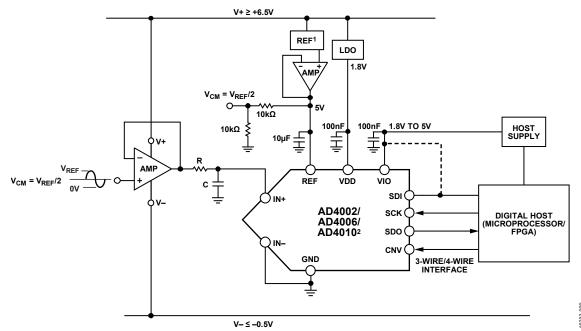
Figure 39. Typical Application Diagram with Multiple Supplies
