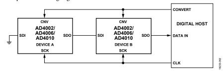
Figure 63. Daisy-Chain Mode, Connection Diagram
