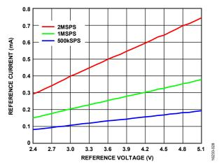
Figure 33. Reference Current vs. Reference Voltage
