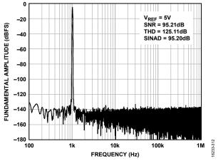
Figure 12. 1 kHz, -0.5 dBFS Input Tone Fast Fourier Transform (FFT),  $V_{\it REF} = 5~V$
