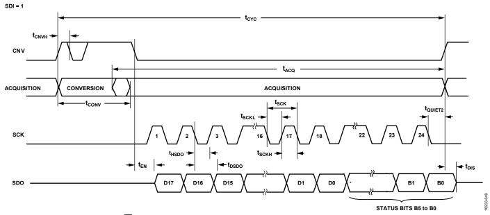
Figure 50. CS Mode, 3-Wire Without Busy Indicator Serial Interface Timing Diagram, Including Status Bits
