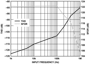
Figure 20. THD and SFDR vs. Input Frequency
