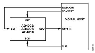
Figure 51. CS Mode, 3-Wire Turbo Mode Connection Diagram
