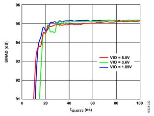
Figure 24. SINAD vs. tQUIET2
