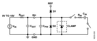
Figure 41. Equivalent Analog Input Circuit
