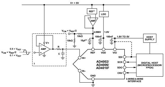
1SEE THE VOLTAGE REFERENCE INPUT SECTION FOR REFERENCE SELECTION. C<sub>REF</sub> IS USUALLY A 10µF CERAMIC CAPACITOR (X7R). 2SPAN COMPRESSION MODE ENABLED. 3SEE TABLE 10 FOR RC FILTER AND AMPLIFIER SELECTION.
