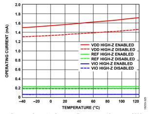
Figure 31. Operating Current vs. Temperature, AD4010, 500 kSPS
