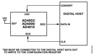
Figure 53. CS Mode, 3-Wire Without Busy Indicator Connection Diagram
