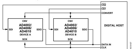
Figure 59. CS Mode, 4-Wire Without Busy Indicator Connection Diagram
