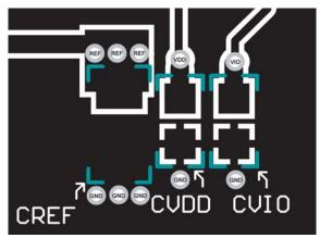
Figure 66. Example Layout of the AD4002 (Bottom Layer)
