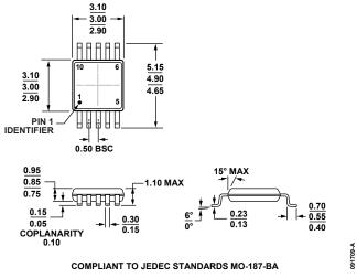
Figure 67. 10-Lead Mini Small Outline Package [MSOP] (RM-10) Dimensions shown in millimeters
