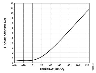
Figure 35. Standby Current vs. Temperature
