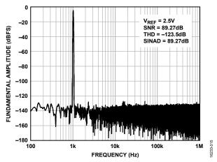
Figure 15. 1 kHz, -0.5 dBFS Input Tone FFT,  $V_{REF} = 2.5$  V
