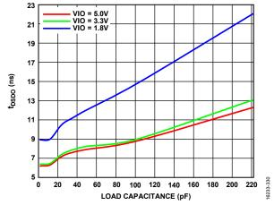
Figure 36.  $t_{DSDO}$  vs. Load Capacitance
