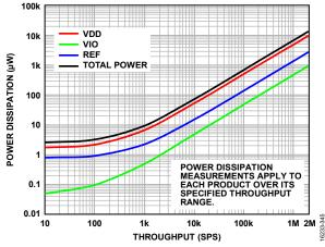
Figure 34. Power Dissipation vs. Throughput, VDD = 1.8 V, VIO = 1.8 V,  $V_{REF} = 5 \text{ V}$
