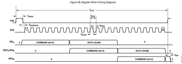
Figure 49. Register Write Timing Diagram, Daisy-Chain Mode
