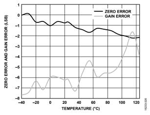
Figure 27. Zero Error and Gain Error vs. Temperature
