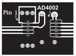
Figure 65. Example Layout of the AD4002 (Top Layer)
