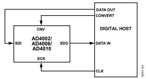
Figure 57. CS Mode, 4-Wire Turbo Mode Connection Diagram
