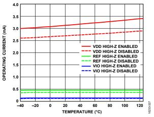
Figure 30. Operating Current vs. Temperature, AD4006, 1 MSPS
