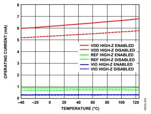
Figure 29. Operating Current vs. Temperature, AD4002, 2 MSPS
