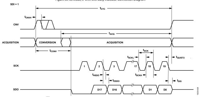
Figure 56. CS Mode, 3-Wire with Busy Indicator Serial Interface Timing Diagram (Status Bits Not Shown)
