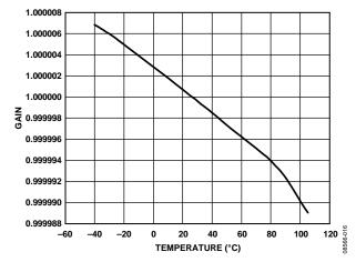
Figure 16. Gain vs. Temperature (Gain = 1)
