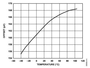
Figure 14. Offset vs. Temperature (Gain = 1, Chop Disabled)
