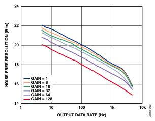
Figure 18. Noise-Free Resolution (Sinc<sup>4</sup> Filter, Chop Disabled,  $V_{REF} = 5 V$ )
