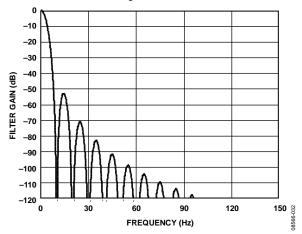
Figure 33. Sinc⁴ Filter Response (FS[9:0] = 480)
