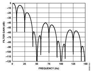
Figure 51. Sinc<sup>3</sup> Filter Response (FS[9:0] = 96, Chop Enabled)
