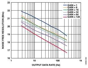
Figure 20. Noise-Free Resolution in Fast Settling Mode ( $V_{REF} = 5 V$ , Averaging by 16, Sinc<sup>4</sup> Filter, Chop Disabled)
