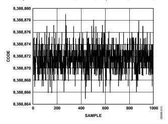
Figure 10. Noise ( $V_{REF} = AV_{DD} = 5 V$ , Output Data Rate = 42.1 Hz (FS[9:0] = 6, Average by 16), Gain = 1, Chop Disabled, Sinc<sup>4</sup> Filter)
