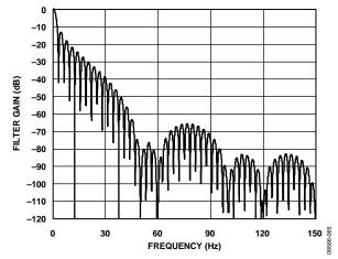
Figure 66. Filter Response for Average + Decimate Filter (Sinc<sup>3</sup> Filter, FS[9:0] = 96, Average by 16)
