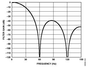
Figure 40. Sinc<sup>3</sup> Filter Response (FS[9:0] = 80)
