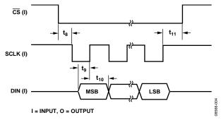
Figure 4. Write Cycle Timing Diagram
