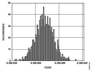
Figure 9. Noise Distribution Histogram ( $V_{REF} = AV_{DD} = 5 V$ , Output Data Rate = 2400 Hz, Gain = 1, Chop Disabled, Sinc<sup>4</sup> Filter)
