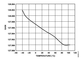
Figure 17. Gain vs. Temperature (Gain = 128)
