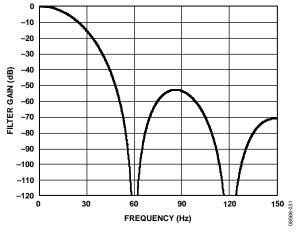
Figure 32. Sinc<sup>4</sup> Filter Response (FS[9:0] = 80)
