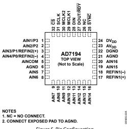
Figure 5. Pin Configuration
