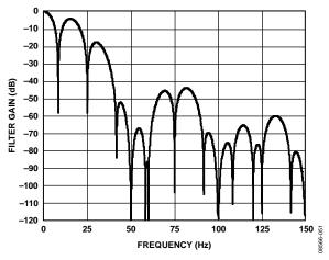
Figure 52. Sinc<sup>3</sup> Filter Response (FS[9:0] = 96, Chop Enabled, REJ60 = 1)
