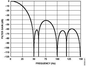
Figure 42. Sinc<sup>3</sup> Filter Response (FS[9:0] = 96, REJ60 = 1)
