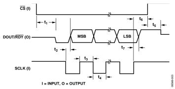
Figure 3. Read Cycle Timing Diagram
