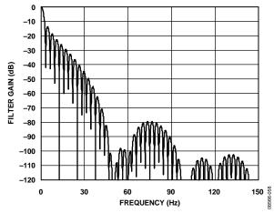
Figure 59. Filter Response for Average + Decimate Filter (Sinc⁴ Filter, FS[9:0] = 96, Average by 16)
