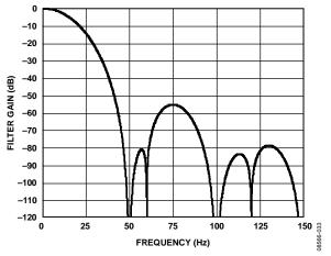
Figure 34.  $Sinc^4$  Filter Response (FS[9:0] = 96, REJ60 = 1)
