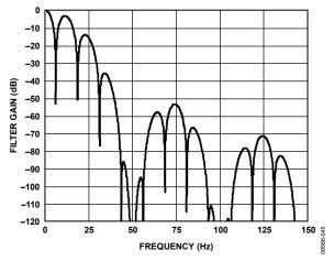
Figure 46. Sinc<sup>4</sup> Filter Response (FS[9:0] = 96, Chop Enabled)
