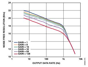
Figure 19. Noise-Free Resolution (Sinc<sup>3</sup> Filter, Chop Disabled,  $V_{REF} = 5 V$ )
