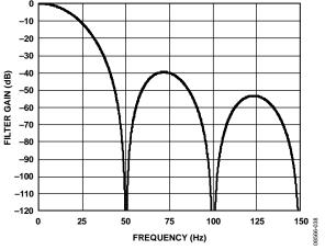
Figure 39.  $Sinc^3$  Filter Response (FS[9:0] = 96)
