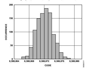
Figure 11. Noise Distribution Histogram ( $V_{REF} = AV_{DD} = 5V$ , Output Data Rate = 42.1 Hz (FS[9:0] = 6, Average by 16), Gain = 1, Chop Disabled, Sinc<sup>4</sup> Filter)
