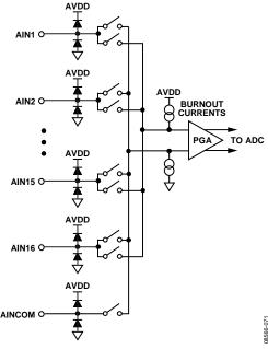
Figure 22. Analog Input Multiplexer Circuit
