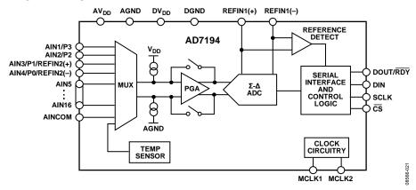
Figure 21. Basic Connection Diagram
