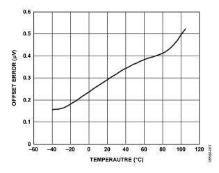
Figure 15. Offset vs. Temperature (Gain = 128, Chop Disabled)
