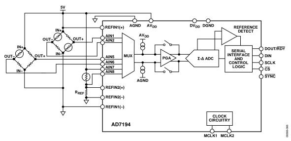
Figure 67. Typical Application (Flowmeter)
