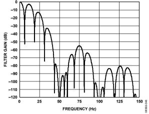
Figure 47. Sinc<sup>4</sup> Filter Response (FS[9:0] = 96, Chop Enabled, REJ60 = 1)
