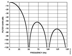
Figure 31. Sinc⁴ Filter Response (FS[9:0] = 96)
