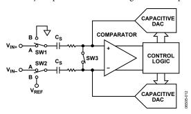
Figure 14. ADC Acquisition Phase
