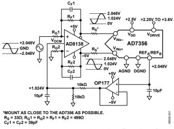
Figure 20. Using the AD8138 as a Single-Ended-to-Differential Amplifier
