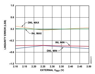
Figure 11. Linearity Error vs. External  $V_{REF}$
