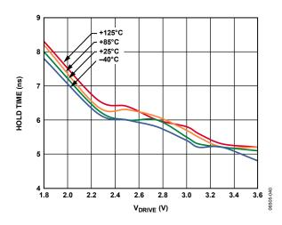
Figure 13. Hold Time vs. V<sub>DRIVE</sub>
