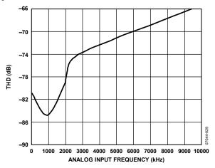
Figure 18. THD vs. Analog Input Frequency
