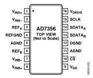
Figure 2. Pin Configuration
