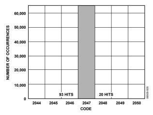
Figure 6. Histogram of Codes for 65,000 Samples
