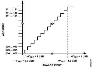
Figure 23. AD7356 Ideal Transfer Characteristic
