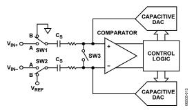
Figure 15. ADC Conversion Phase
