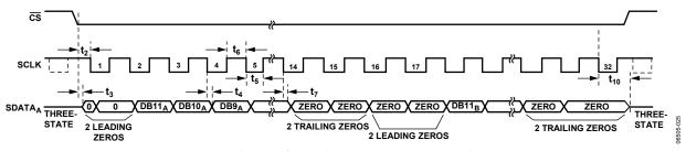
Figure 31. Reading Data from Both ADCs on One SDATA Line with 32 SCLKs
