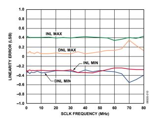
Figure 10. Linearity Error vs. SCLK Frequency
