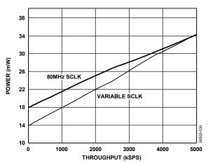
Figure 29. Power vs. Throughput Rate
