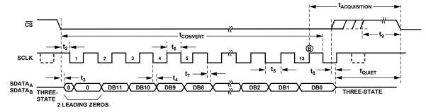
Figure 30. Serial Interface Timing Diagram
