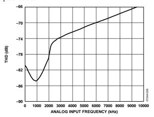
Figure 18. THD vs. Analog Input Frequency
