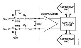
Figure 14. ADC Acquisition Phase
