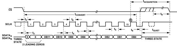
Figure 30. Serial Interface Timing Diagram
