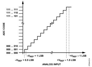
Figure 23. AD7352 Ideal Transfer Characteristic
