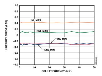
Figure 10. Linearity Error vs. SCLK Frequency
