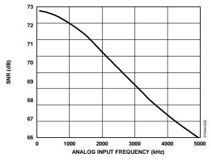
Figure 7. SNR vs. Analog Input Frequency
