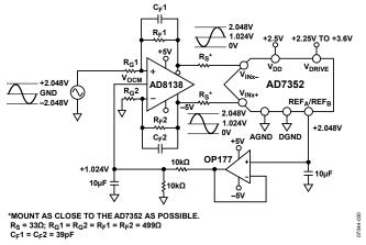
Figure 20. Using the AD8138 as a Single-Ended-to-Differential Amplifier
