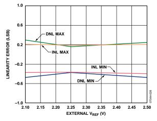
Figure 11. Linearity Error vs. External V<sub>REF</sub>
