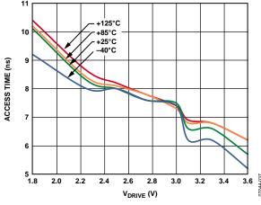
Figure 12. Access Time vs. V<sub>DRIVE</sub>
