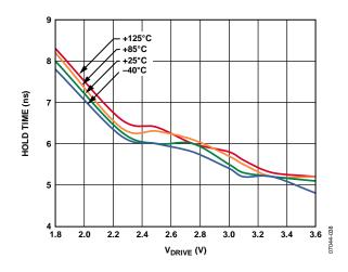
Figure 13. Hold Time vs. V<sub>DRIVE</sub>
