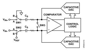
Figure 15. ADC Conversion Phase
