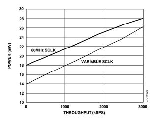
Figure 29. Power vs. Throughput Rate
