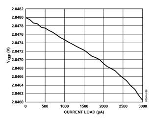
Figure 9. V<sub>REF</sub> vs. Reference Output Current Drive
