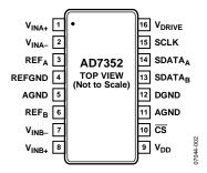
Figure 2. Pin Configuration
