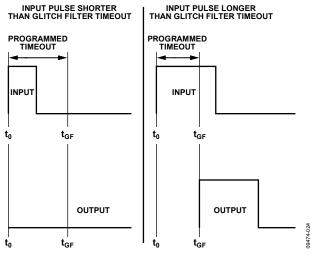
Figure 15. Input Glitch Filter Function
