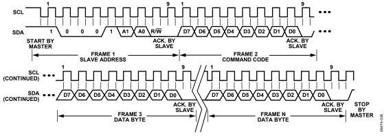
Figure 25. General SMBus Write Timing Diagram
