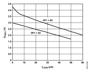
Figure 12. V<sub>PDO1</sub> (Weak Pull-Up to VPx) vs. I<sub>LOAD</sub>
