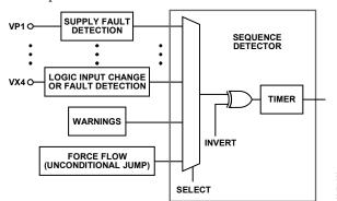
Figure 20. Sequence Detector Block Diagram
