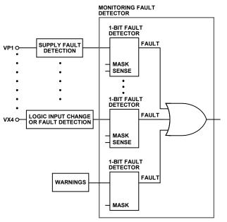
Figure 22. Monitoring Fault Detector Block Diagram
