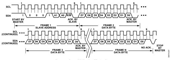
Figure 26. General SMBus Read Timing Diagram
