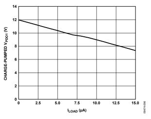
Figure 10. Charge-Pumped V<sub>PDO1</sub> (FET Drive Mode) vs. I<sub>LOAD</sub>
