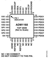
Figure 3. Pin Configuration
