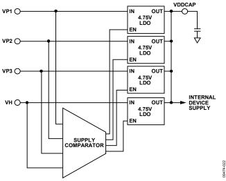
Figure 14. V<sub>DD</sub> Arbitrator Operation
