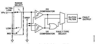
Figure 16. Supply Fault Detector Block
