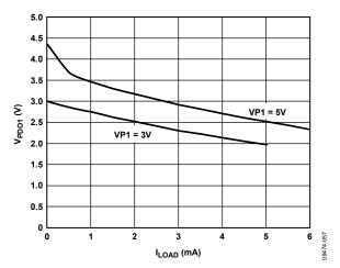
Figure 11. V<sub>PDO1</sub> (Strong Pull-Up to VPx) vs. I<sub>LOAD</sub>
