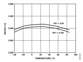
Figure 13. REFOUT vs. Temperature
