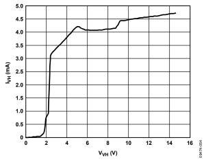
Figure 8. I<sub>VH</sub> vs. V<sub>VH</sub> (VH as Supply)
