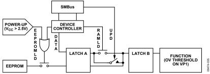
Figure 24. Configuration Update Flow Diagram
