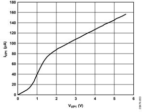
Figure 7. I<sub>VP1</sub> vs. V<sub>VP1</sub> (VP1 Not as Supply)
