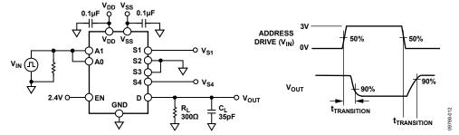
Figure 29. Address to Output Switching Times
