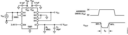
Figure 30. Break-Before-Make Time Delay, t<sub>D</sub>
