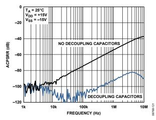
Figure 20. ACPSRR vs. Frequency, ±15 V Dual Supply
