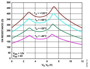
Figure 10.  $R_{ON}$  as a Function of  $V_D$  or  $V_S$  for Different Temperatures, 12 V Single Supply
