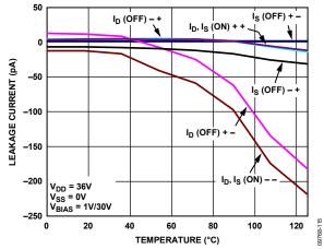
Figure 15. Leakage Current vs. Temperature, 36 V Single Supply
