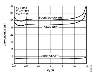
Figure 21. Capacitance vs. Source Voltage, Dual Supply
