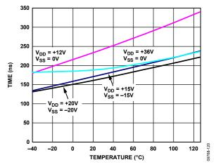
Figure 19. Transition Time vs. Temperature
