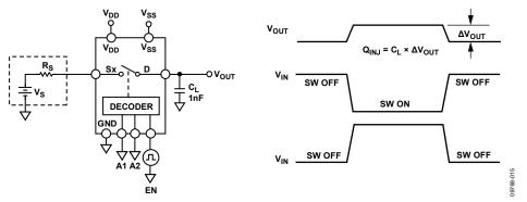
Figure 32. Charge Injection
