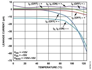
Figure 12. Leakage Current vs. Temperature, ±15 V Dual Supply
