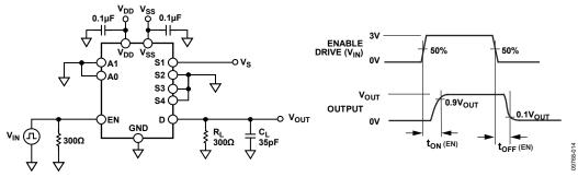
Figure 31. Enable-to-Output Switching Delay
