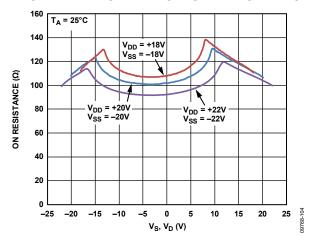
Figure 4.  $R_{ON}$  as a Function of  $V_D$  or  $V_S$ , Dual Supply
