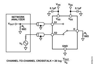
Figure 28. Channel-to-Channel Crosstalk
