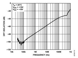
Figure 16. Off Isolation vs. Frequency, ±15 V Dual Supply
