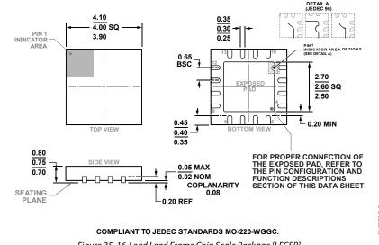
Figure 35. 16-Lead Lead Frame Chip Scale Package [LFCSP] 4 mm × 4 mm Body and 0.75 mm Package Height (CP-16-17) Dimensions shown in millimeters
