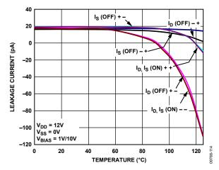
Figure 14. Leakage Current vs. Temperature, 12 V Single Supply
