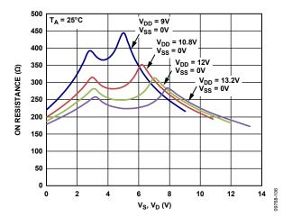
Figure 6.  $R_{ON}$  as a Function of  $V_D$  or  $V_S$ , Single Supply
