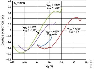
Figure 18. Charge Injection vs. Source Voltage
