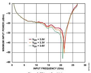
Figure 3. RF Input Sensitivity
