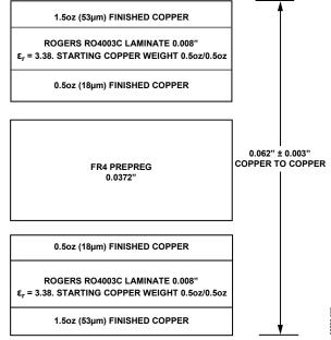
Figure 9. Evaluation Board PCB Layer Stack-Up
