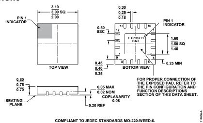
Figure 11. 16-Lead Lead Frame Chip Scale Package [LFCSP\_WQ] 3 mm × 3 mm Body, Very Very Thin Quad (CP-16-18) Dimensions shown in millimeters
