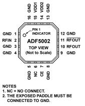
Figure 2. Pin Configuration
