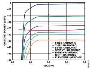
Figure 6. RF Output Harmonic Content vs. VDDx
