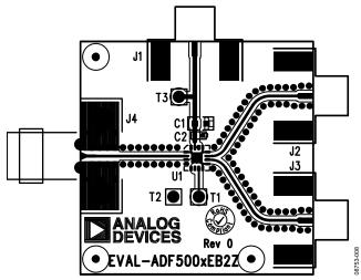
Figure 8. Evaluation Board Silkscreen—Top View
