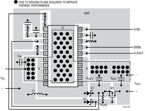
A- RETURN  $\rm C_{IN}$  ground directly to 1t3579 exposed PAD PIN 21. It is advised to not combine  $\rm C_{IN}$  ground with gnd except at the exposed PAD.
