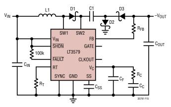
Figure 15. Single Inductor Inverting Topology
