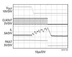
Figure 4. Output Short Circuit Protection of the LT3579
