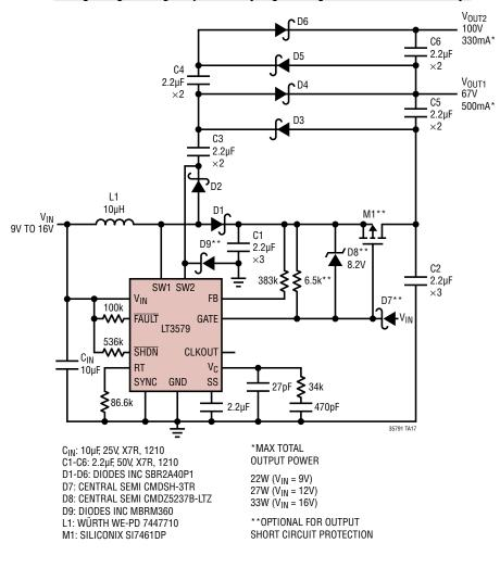
VFD (Vacuum Fluorescent Display) Power Supply Switches at 1MHz Danger High Voltage! Operation by High Voltage Trained Personnel Only
