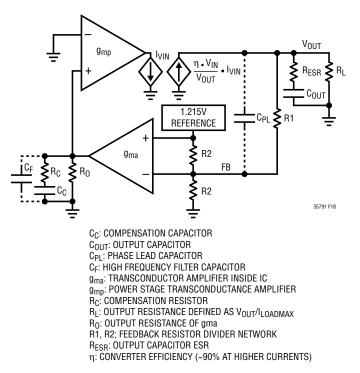
Figure 18. Boost Converter Equivalent Model
