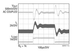
Figure 17a. Transient Response Shows Excessive Ringing
