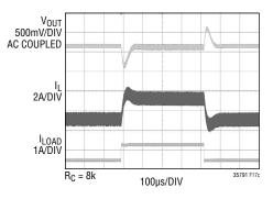
Figure 17c. Transient Response Is Well Damped
