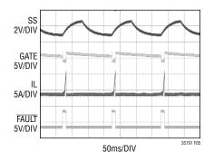
Figure 5. Continuous Output Short Showing FAULT Timeout Cycle
