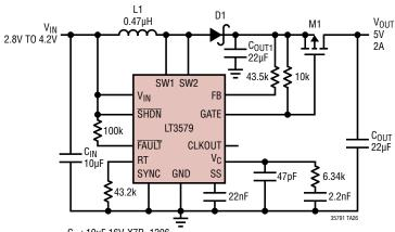
С<sub>IN</sub>: 10µF, 16V, X7R, 1206 С<sub>ОUT1</sub>, С<sub>OUT</sub>: 22µF, 16V, X7R, 1210 D1: CENTRAL SEMI CTLSH3-30M833 L1: VISHAY IHLP-2020BZ-01-R47 M1: SILICONIX SI7123DN
