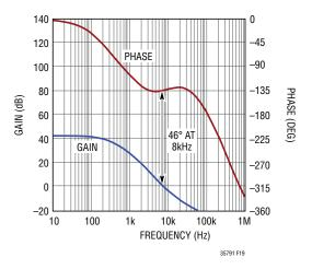
Figure 19. Bode Plot for Example Boost Converter
