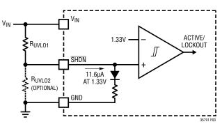
Figure 3. Configurable UVLO
