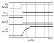
Figure 14.  $V_{\text{IN}}$  Hot-Plug Control. Inrush Current is Well Controlled
