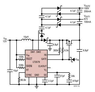
Figure 16. High V<sub>OUT</sub> Charge Pump Topology
