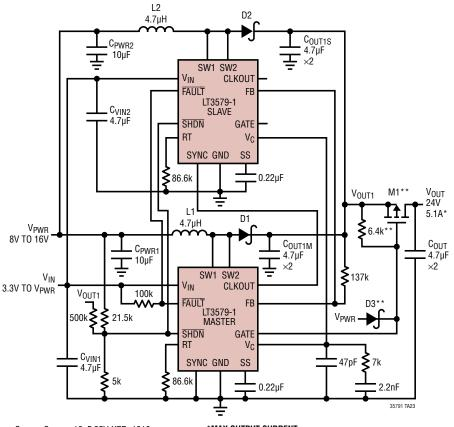
1MHz, 2-Phase Converter Generates a 24V Output from a 8V to 16V Input and Uses Small Components
