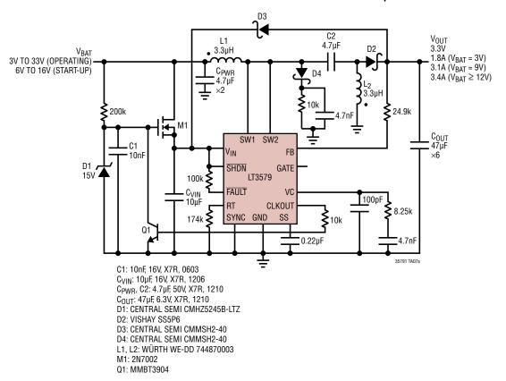
500kHz SEPIC Converter Generates 3.3V from a 3V to 33V Input
