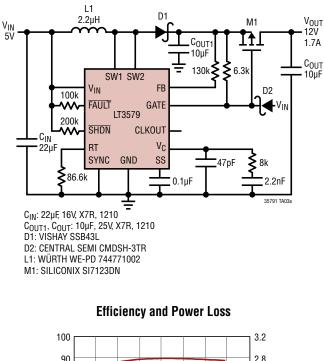
1MHz, 5V to 12V Boost Converter can Survive Output Shorts
