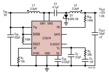
Figure 8. Dual Inductor Inverting Converter – The Component Values Given Are Typical Values for a 1.2MHz, 5V to –12V Inverting Topology Using Coupled Inductors
