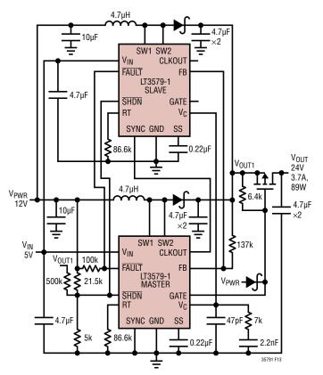
Figure 13. 2-Phase Converters Using LT3579-1
