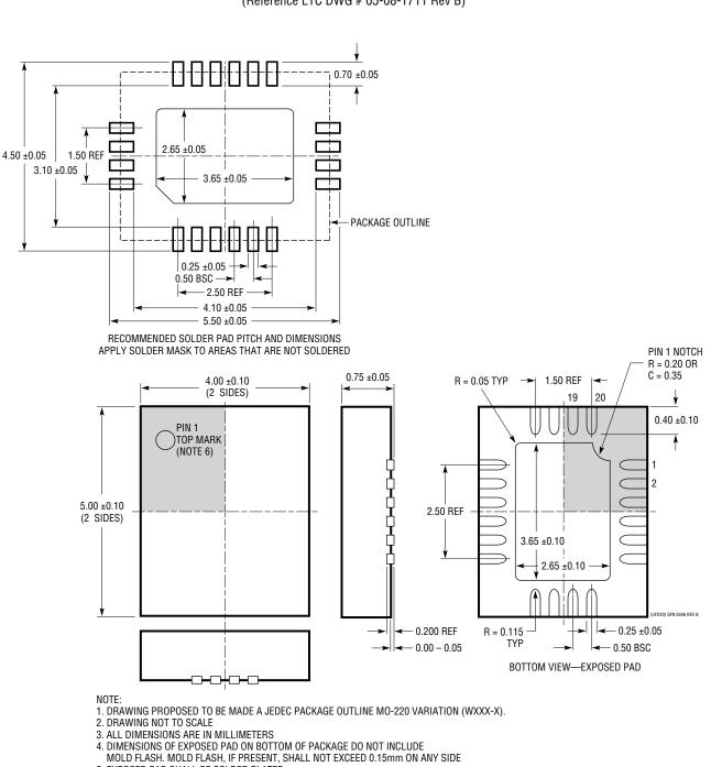
**UFD Package** 20-Lead Plastic QFN ( $4mm \times 5mm$ )
