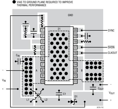
A- RETURN C<sub>IN</sub> AND L2 GROUND DIRECTLY TO LT3579 EXPOSED PAD PIN 21. IT IS ADVISED TO NOT COMBINE C<sub>IN</sub> AND L2 GROUND WITH GND EXCEPT AT THE EXPOSED PAD. B- RETURN C<sub>OUT</sub> GROUND DIRECTLY TO LT3579 EXPOSED PAD PIN 21. IT IS ADVISED TO NOT COMBINE C<sub>OUT</sub> GROUND WITH GND EXCEPT AT THE EXPOSED PAD. L1, L2 -MOST COUPLED INDUCTOR MANUFACTURERS USE CROSS PINOUT FOR IMPROVED PERFORMANCE.
