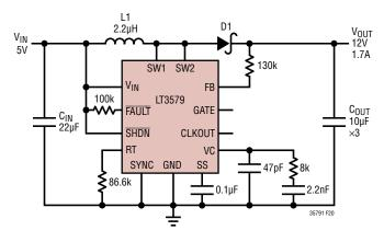
Figure 20. 5V to 12V Boost Converter
