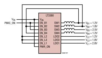
Figure 7. Pin-Strapped Power-On Sequence Application
