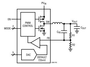
Figure 2. Step-Down Switching Regulator Application Circuit
