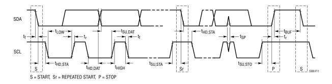
Figure 11. LT3380 I<sup>2</sup>C Serial Port Timing
