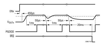
Figure 10. Output Low Voltage PGOOD and IRQ Timing
