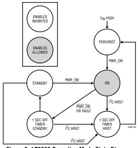
Figure 5. LT3380 Operating Mode State Diagram
