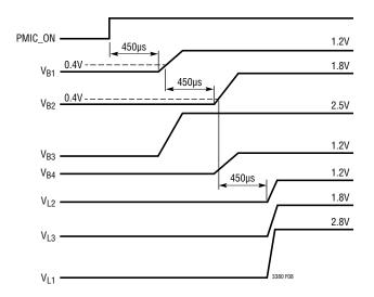
Figure 8. Pin-Strapped Power-On Sequence
