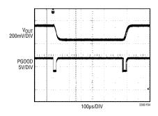
Figure 4. Dynamic Voltage Scaling
