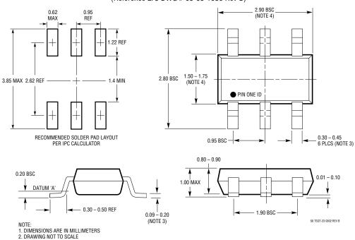
2. DRAWING NOT TO SCALE 3. DIMENSIONS ARE INCLUSIVE OF PLATING 4. DIMENSIONS ARE EXCLUSIVE OF MOLD FLASH AND METAL BURR 5. MOLD FLASH SHALL NOT EXCEED 0.254mm
