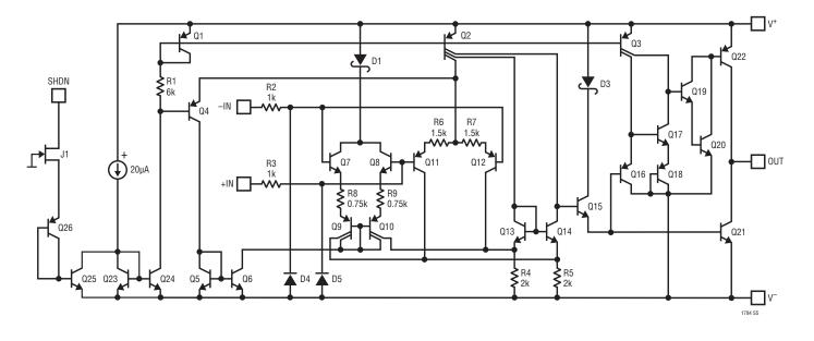
the SHDN pin 1.2V or more above V<sup>-</sup>. When shut down, the supply current is less than 1µA (V<sup>-</sup>  $\leq$  V<sub>OUT</sub>  $\leq$  V<sup>+</sup>). In normal operation, the SHDN pin can be tied to V<sup>-</sup> or left floating. See Typical Performance Characteristics curve, "Supply Current vs SHDN pin Voltage."
