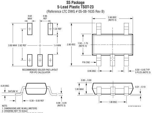
2. DRAWING NOT 10 SCALE 3. DIMENSIONS ARE INCLUSIVE OF PLATING 4. DIMENSIONS ARE EXCLUSIVE OF MOLD FLASH AND METAL BURR 5. MOLD FLASH SHALL NOT EXCEED 0.2854mm 6. JEDEC PACKAGE REFERENCE IS M0-193
