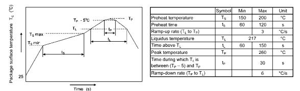
• The soldering temperature profile is based on the package surface temperature (See the figure shown below, which is based on the package surface temperature.)
