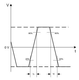
Figure 8. LVDS Differential Waveform (i.e. OUT+ minus OUT-)
