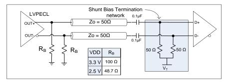
Figure 11. LVPECL with AC-coupled termination
