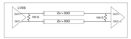
Figure 17. LVDS double DC termination
