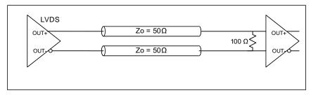
Figure 15. LVDS single DC termination at the load
