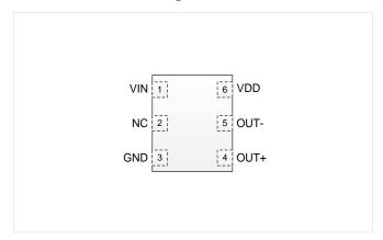
Figure 2. Pin Assignments (Top view)
