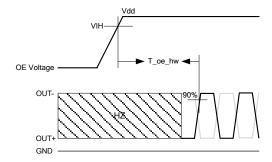
Figure 9. Hardware OE Enable Timing
