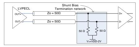
Figure 14. LVPECL with DC-coupled parallel shunt load termination
