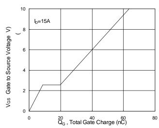
Fig.4 Gate-Charge Characteristics
