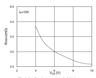
Fig.2 On-Resistance vs. G-S Voltage
