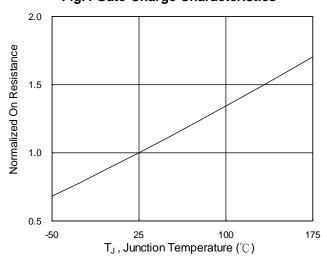
Fig.6 Normalized R<sub>DSON</sub> vs. T<sub>J</sub>
