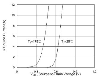
Fig.3 Forward Characteristics of Reverse
