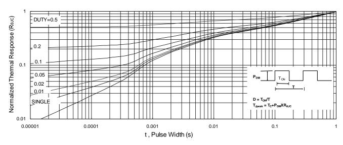
Fig.9 Normalized Maximum Transient Thermal Impedance
