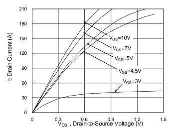
**Fig.1 Typical Output Characteristics**
