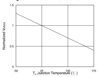
Fig.5 Normalized V<sub>GS(th)</sub> vs. T<sub>J</sub>
