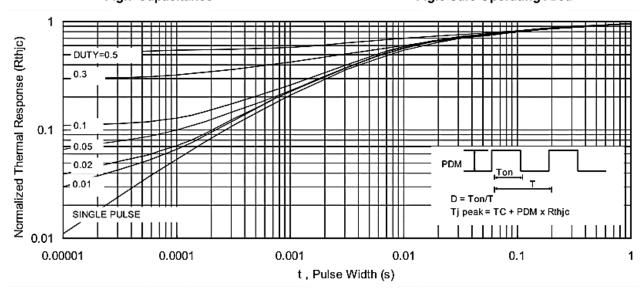
Fig.9 Normalized Maximum Transient Thermal Impedance
