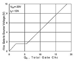
Fig.4 Gate-Charge Characteristics
