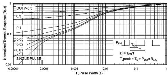
Fig.9 Normalized Maximum Transient Thermal Impedance
