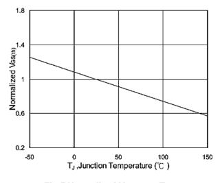
Fig.5 Normalized V<sub>GS(th)</sub> v.s T<sub>J</sub>
