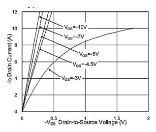
Fig.1 Typical Output Characteristics
