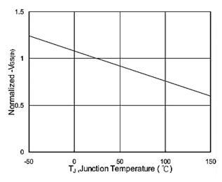
Fig.5 Normalized V<sub>GS(th)</sub> v.s T<sub>J</sub>
