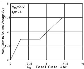
Fig.4 Gate-Charge characteristics
