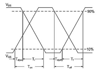
Fig.10 Switching Time Waveform
