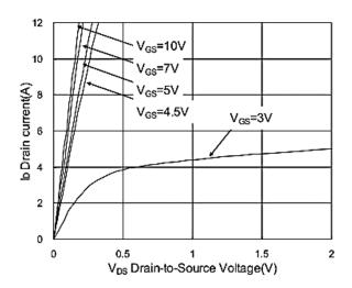
Fig.1 Typical Output Characteristics
