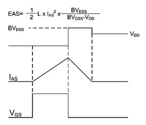
Fig.11 Unclamped Inductive Waveform
