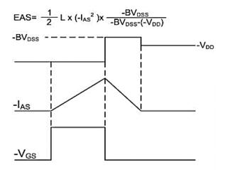
Fig.11 Unclamped Inductive Waveform
