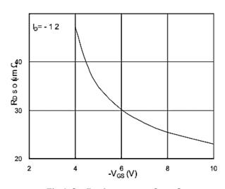
Fig.2 On-Resistance v.s Gate-Source
