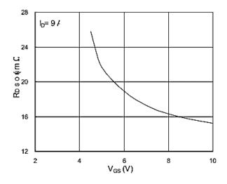
Fig.2 On-Resistance v.s Gate-Source
