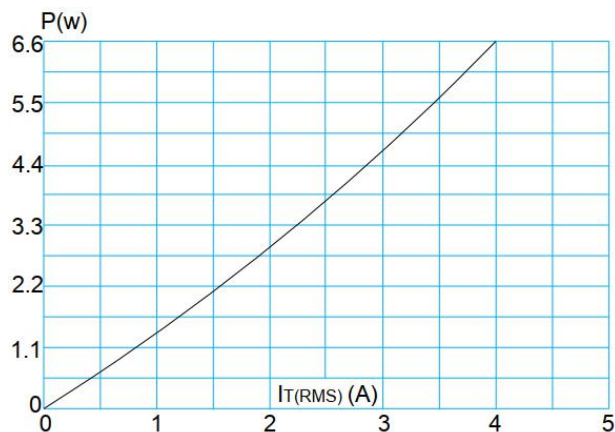
FIG.1: Maximum power dissipation versus RMS on-state current
