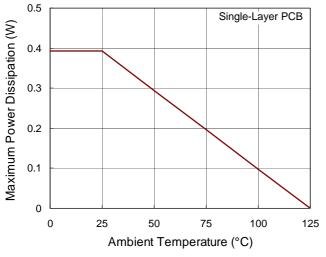
Figure 7. Derating Curves for RT8514 Package
