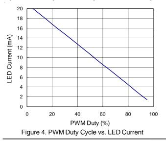
By the above equation and the application circuit shown in Figure 3, and assume the RT8514 is selected which  $V_{REF}$  is equal to 0.3V. Figure 4 shows the relationship between the LED current and PWM duty cycle. For example, when the PWM duty is equal to 60%, the LED current will be equal to 8.6mA. When the PWM duty is equal to 40%, the LED current will be equal to 12.7mA.
