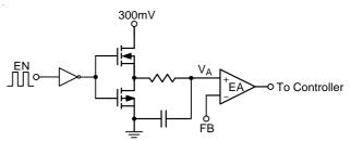
Figure 1. Block Diagram of Programmable FB Voltage Using PWM Signal
