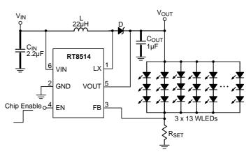
Figure 6. Application for Driving 3 X 13 WLEDs
