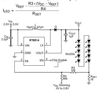
Figure 2. Dimming Control Using a DC Voltage
