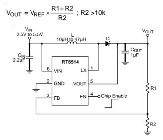
Figure 5. Constant Output Voltage Application
