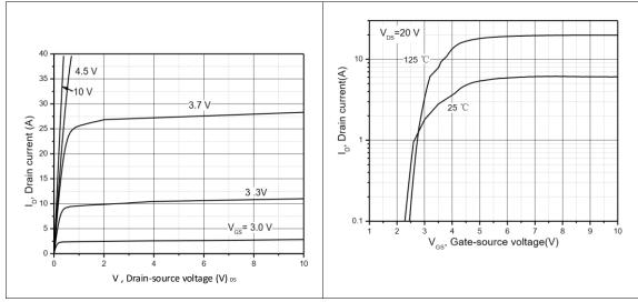
Figure 1, Typ. output characteristics
