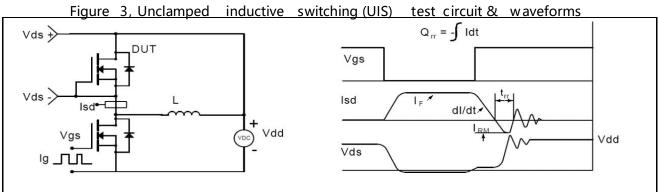
Figure 4, Diode reverse recovery test circuit & waveforms
