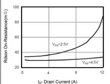
Figure 6 Drain-Source On-Resistance
