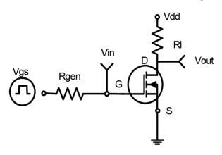
Figure 1:Switching Test Circuit
