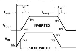
Figure 2:Switching Waveforms
