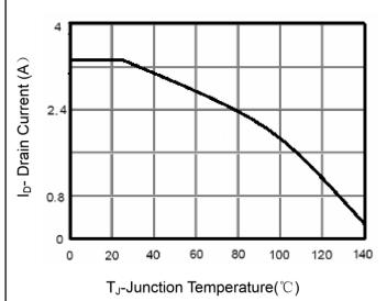
**Figure 4 Drain Current**
