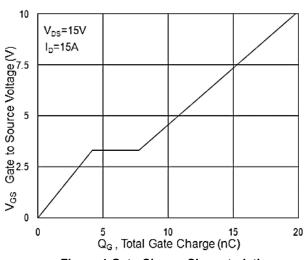
Figure 4: Gate-Charge Characteristics
