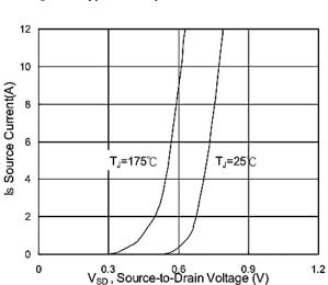
Figure3:Forward Characteristics of Reverse diode
