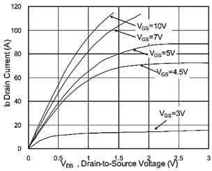
Figure1:Typical Output Characteristics
