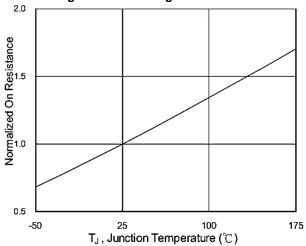
Figure6: Normalized R DSON vs. T J
