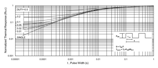
Figure9: Normalized Maximum Transient Thermal Impedance
