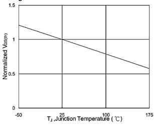
Figure 5: Normalized V GS(th) vs. T J
