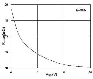
Figure2:On-Resistance vs. G-S Voltage
