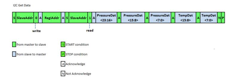
For Pressure data only, the data stream can be terminated after the sixth pressure byte. See Figure 2 below.
