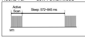
Note: If the device makes a proximity or touch detection, it will automatically perform active scans continually. Once the device releases from its proximity-detected state, it will return to the power mode set by the MTPM pin.
