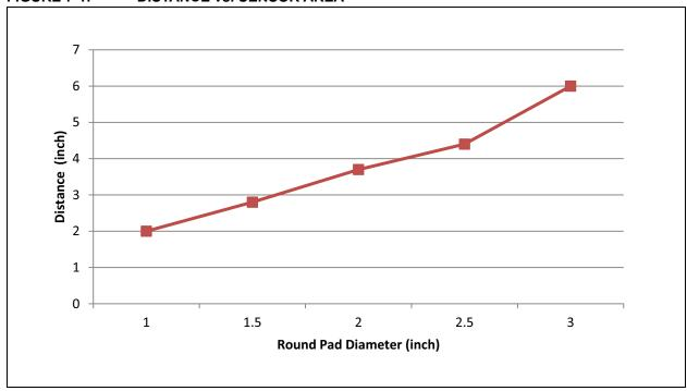
**Note:** The tested sensors are round solid pads on FR4 PCB. No ground plane was near the sensor, as this would give the maximum detection distance.
