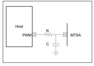
Note 1: Application Note AN538, "Using PWM to Generate Analog Output" has details about how to choose appropriate R and C values.
