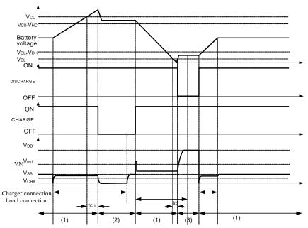
Figure 5-1 Overcharge and Overdischarge Voltage Detection
