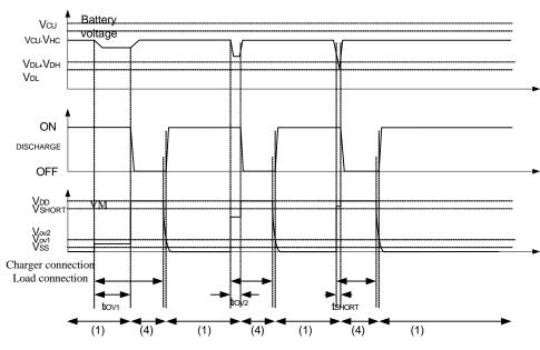
Figure 5-2 Overdischarge Current Detection
