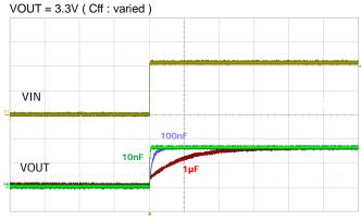
VIN: 2.0V/div, VOUT: 2.0V/div, Time: 50ms/div Start Up @ Iout=10mA
