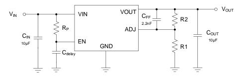
Fig. 3. Application with Delayed Start-Up
