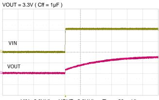
$\label{eq:VIN:2.0V/div} VIN: 2.0V/\text{div}, \quad \text{Vout: 2.0V/div}, \quad \text{Time: 20ms/div} \\ Start \ Up \ @ \ Iout=0A$
