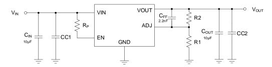
Fig. 2. Application with Feed-Forward Capacitor, CFF
