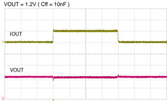
IOUT : 1.0A/div, VOUT : 100mV/div, Time : 500μs/div Load Transient Response
