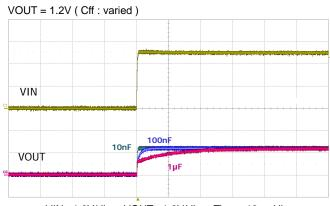
VIN: 1.0V/div, VOUT: 1.0V/div, Time: 10ms/div Start Up @ Iout=10mA
