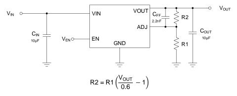
Fig. 4. Application for Adjustable Output Voltage
