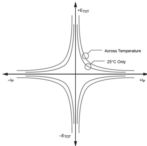
Figure 3: Total Output Error versus Sensed Current
