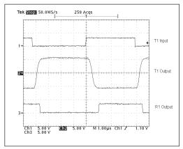
Figure 12. Loopback Test results at 250kbps
