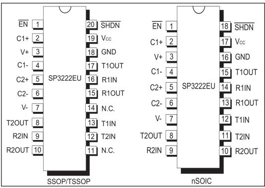
Figure 7. Pinout Configurations for the SP3222EU
