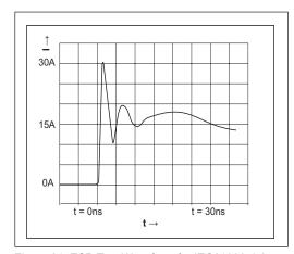
Figure 21. ESD Test Waveform for IEC61000-4-2
