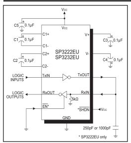
Figure 11. SP3222EU/SP3232EU Driver Loopback Test Circuit
