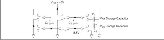
Figure 15. Charge Pump — Phase 2
