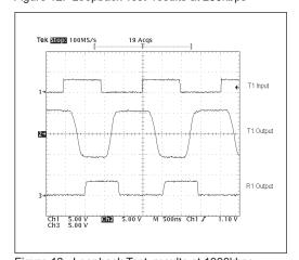
Figure 13. Loopback Test results at 1000kbps
