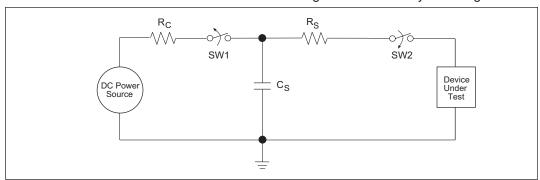
Figure 19. ESD Test Circuit for Human Body Model 205-32xxEUDSR00
