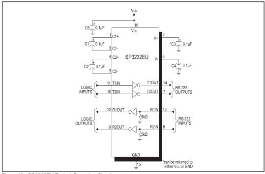
Figure 10. SP3232EU Typical Operating Circuit
