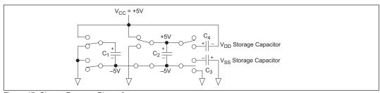
Figure 17. Charge Pump — Phase 3
