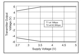
Figure 5. Transmitter Output Voltage vs Supply Voltage for the SP3222EU and SP3232EU
