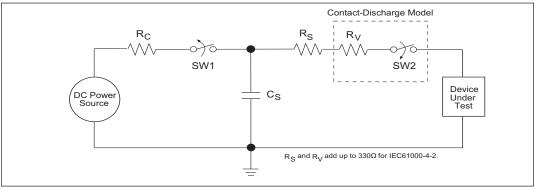
Figure 20. ESD Test Circuit for IEC61000-4-2
