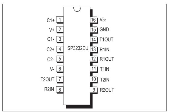
Figure 8. Pinout Configuration for the SP3232EU
