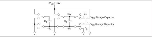
Figure 14. Charge Pump — Phase 1
