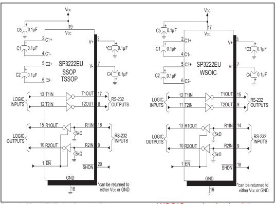
Figure 9. SP3222EU Typical Operating Circuits
