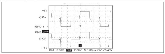
Figure 16. Charge Pump Waveforms
