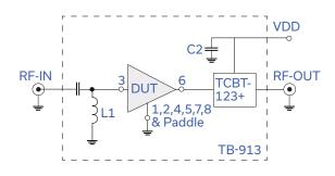
Fig 2. Test board (TB-913+) includes case, connectors and components soldered to PCB. (TB-913+ is a 3-layer PCB. See TB-913+ drawing.)
