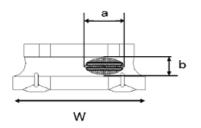
Exposed wire tolerance limit of coating resin part on product side. Size of exposed wire occurring to coating resin is specified below. 1. Width direction (dimension a): Acceptable when  $a \leq w/2$ .
