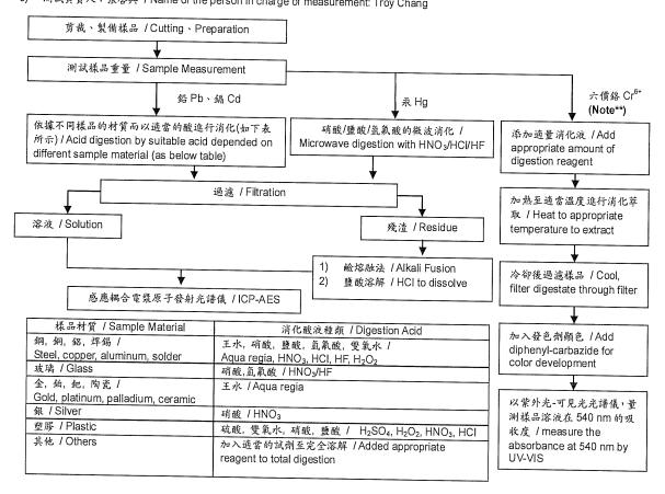
Note\*\*:(1) 針對非金屬材料加入鹼性消化液,加熱至 90~95℃ 萃取. / For non-metallic material, add alkaline digestion reagent and heat to 90~95℃.
