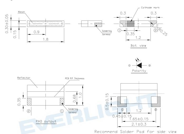
Suggested pad dimension is just for reference only. Please modify the pad dimension based on individual need. Note: Tolerances unless mentioned  $\pm 0.1$ mm. Unit = mm
