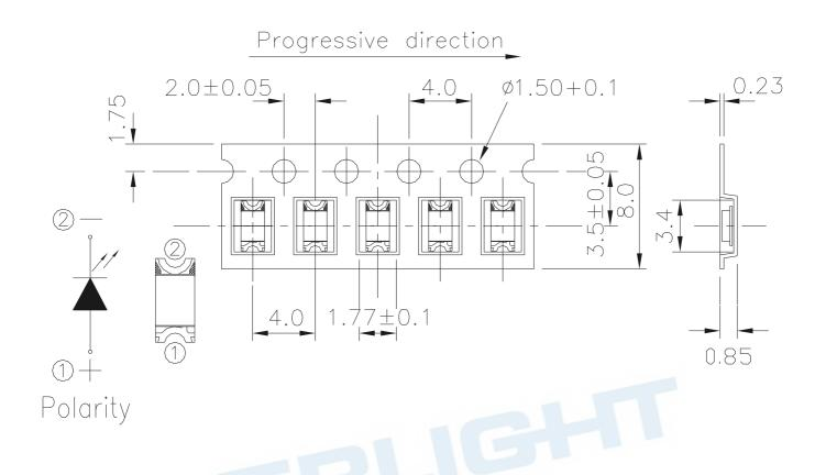
Note: The tolerances unless mentioned is ±0.1mm ,Unit = mm
