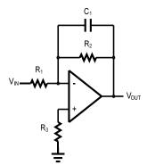
Figure 5. Low Pass Active Filter
