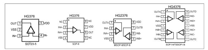
Figure 1. Pin Assignment Diagram
