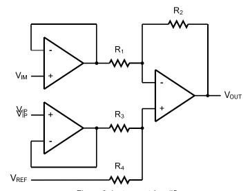
Figure 6. Instrument Amplifier
