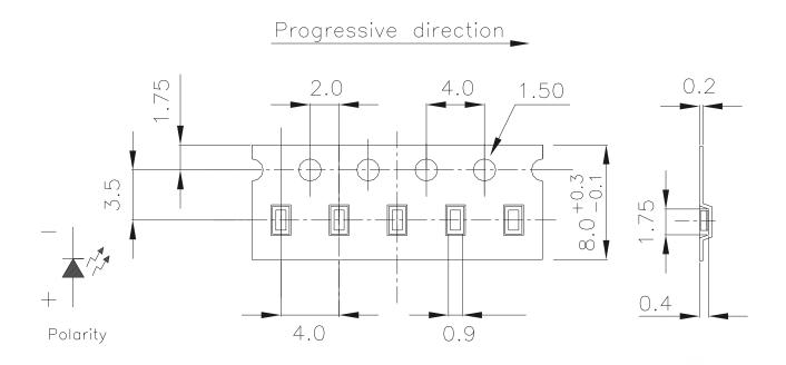
Note: The tolerances unless mentioned is  $\pm 0.1 \text{mm}$ , Unit = mm
