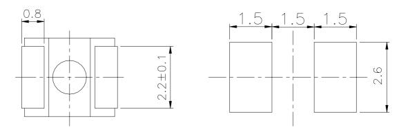
**Note:** The tolerances unless mentioned is  $\pm 0.1$ mm, Unit = mm
