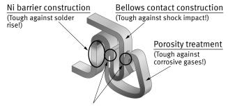
V notch and Double contact constructions
