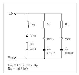
Under normal conditions, when  $I_{SLPE} >> I_{CC} + 0.5 \text{mA} + I_p$ , the static behaviour of the circuit is that of a 3.7V regulator diode with an internal resistance equal to that of R9. In the audio frequency range the dynamic impedance is largely determined by R1. Fig.2 show the equivalent impedance of the circuit.
