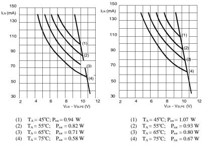
Fig.3a Safe operating area (Standard DIP)
