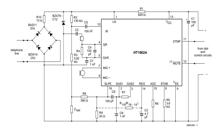
The diode bridge, the Zener diode and R10 limit the current into, and the voltage across, the circuit during line transients.
