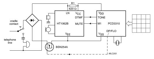
(a) DTMF pulse set with CMOS bilingual dialling circuit PCD3310. The dashed line shows an optional flash (register recall by timed loop break).
