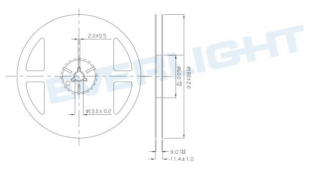
Note: The tolerances unless mentioned is  $\pm 0.1$ mm ,Unit = mm
