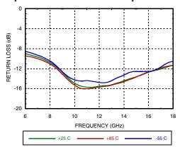
**Output Return Loss vs. Temperature**
