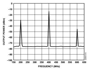
Figure 22. Output Spectrum for Configuration of Figure 21
