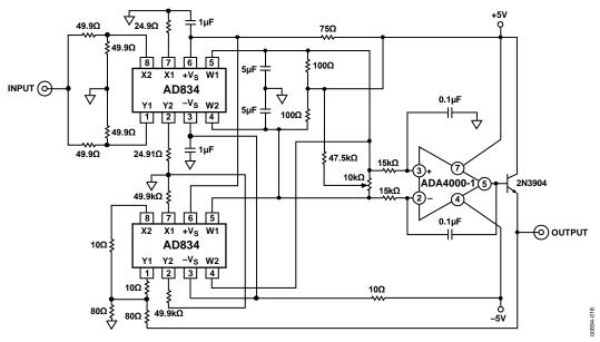
Figure 20. Connections for Wideband RMS Measurement
