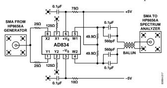
Figure 21. Frequency Doubler Connections
