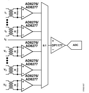
Figure 49. Voltage and Current Monitoring in 3-Phase Power Line Protection Using the AD8276
