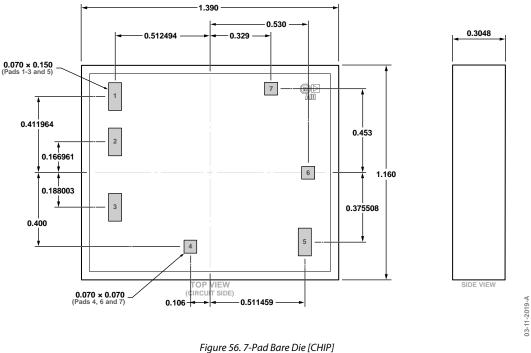
Figure 56. 7-Pad Bare Die [CHIP] (C-7-8) Dimensions shown in millimeters
