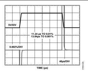
Figure 29. Large Signal Pulse Response and Settling Time, 10 V Step,  $V_{\rm S}=\pm 15$  V
