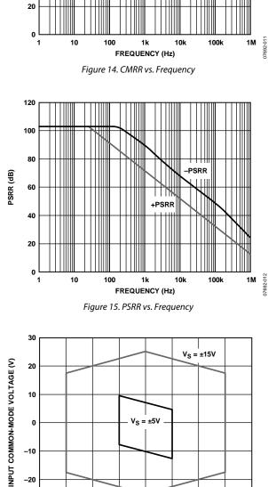
OUTPUT VOLTAGE (V) Figure 16. Input Common-Mode Voltage vs. Output Voltage, ±15 V and ±5 V Supplies
