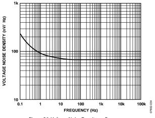
Figure 36. Voltage Noise Density vs. Frequency
