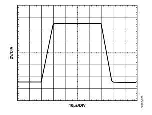
Figure 31. Large Signal Step Response
