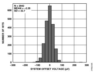
Figure 8. Distribution of Typical System Offset Voltage
