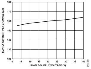
Figure 24. Supply Current Per Channel vs. Single-Supply Voltage,  $V_{IN} = 0 V$ ,  $V_{REF} = 0 V$
