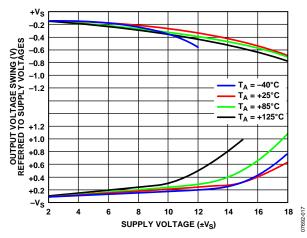
Figure 20. Output Voltage Swing (V) Referred to Supply Voltages vs. Supply Voltage Per Channel and Temperature,  $R_L = 2 k\Omega$
