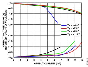
Figure 22. Output Voltage Swing (V) Referred to Supply Voltages vs. Output Current and Temperature,  $V_s = \pm 15 V$
