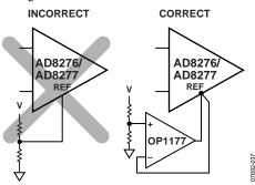
Figure 41. Driving the Reference Pin
