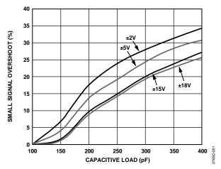
Figure 35. Small Signal Overshoot vs. Capacitive Load,  $R_L \ge 2 k\Omega$
