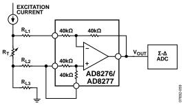
Figure 53. 3-Wire RTD Cable Resistance Error Measurement
