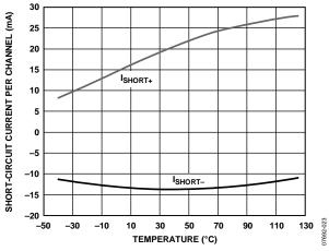
Figure 26. Short-Circuit Current Per Channel vs. Temperature
