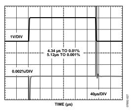
Figure 30. Large Signal Pulse Response and Settling Time, 2 V Step,  $V_{\rm S}$  = 2.7 V
