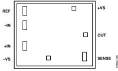
Figure 6. AD8276 7-Pad CHIP Pad Configuration
