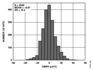
Figure 9. Distribution of Typical Common-Mode Rejection Ratio
