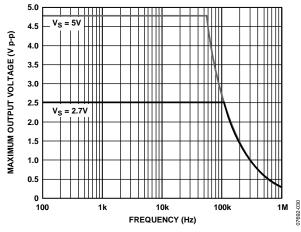
Figure 33. Maximum Output Voltage vs. Frequency,  $V_{\rm S} = 5 V$ , 2.7 V
