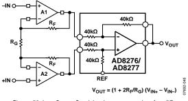
Figure 52. Low Power Precision Instrumentation Amplifier
