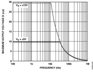
Figure 32. Maximum Output Voltage vs. Frequency,  $V_5 = \pm 15 V$ ,  $\pm 5 V$
