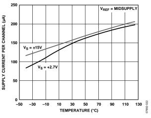
Figure 25. Supply Current Per Channel vs. Temperature
