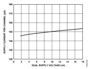
Figure 23. Supply Current Per Channel vs. Dual Supply Voltage,  $V_{IN} = 0 V$
