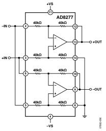
Figure 48. AD8277 Differential Output Configuration
