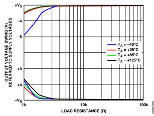
Figure 21. Output Voltage Swing (V) Referred to Supply Voltages vs. Load Resistance and Temperature,  $V_S = \pm 15$  V
