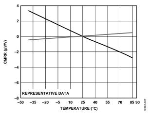
Figure 10. CMRR vs. Temperature, Normalized at 25°C
