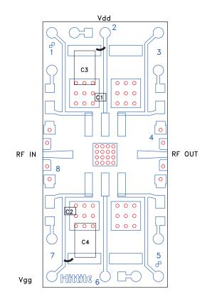
The grounded Co-Planar Wave Guide (CPWG) PCB input/output transitions allow use of Ground-Signal-Ground (GSG) probes for testing. Suggested probe pitch is 400um (16 mils). Alternatively, the board can be mounted in a metal housing with 2.4mm coaxial connectors.
