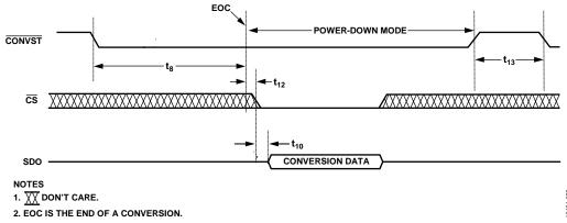
Figure 30. Entering/Exiting Power-Down Mode
