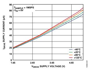
Figure 16. Operational IDRIVE Supply Current vs. VDRIVE Supply Voltage for Various Temperatures
