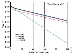
Figure 14. Reference Voltage Output vs. Current Load for Various Temperatures
