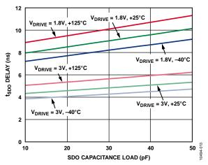
Figure 13. t<sub>SDO</sub> Delay vs. SDO Capacitance Load and V<sub>DRIVE</sub>
