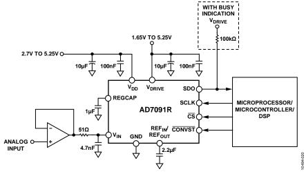
Figure 22. AD7091R Typical Connection Diagram
