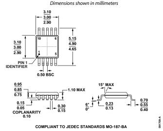
Figure 33. 10-Lead Mini Small Outline Package [MSOP] (RM-10) Dimensions shown in millimeters
