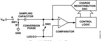
Figure 19. ADC Conversion Phase
