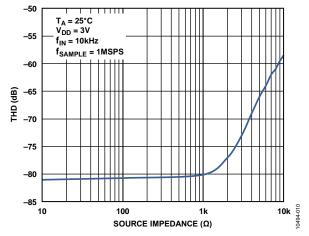
Figure 10. THD vs. Source Impedance
