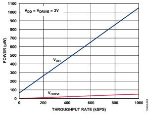
Figure 2. Power vs. Throughput Rate
