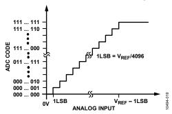
Figure 20. AD7091R Ideal Transfer Characteristics
