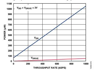
Figure 23. Power Dissipation vs. Throughput Rate (Full Range)
