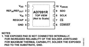
Figure 3. Pin Configuration, 10-Lead LFCSP
