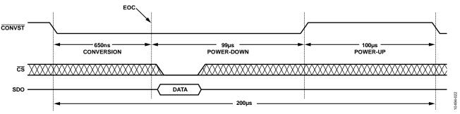
Figure 25. 10 SPS with Normal and Power-Down Mode
