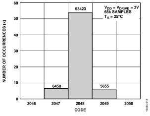
Figure 12. Histogram of Codes at Code Center (V<sub>REF</sub>/2)
