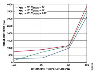
Figure 17. Total Power-Down Supply Current (I<sub>DD</sub> and I<sub>DRIVE</sub>) vs. Temperature for Various Supply Voltages
