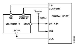
Figure 26. Connection Diagram with BUSY Indicator
