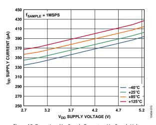
Figure 15. Operational  $I_{DD}$  Supply Current vs.  $V_{DD}$  Supply Voltage for Various Temperatures
