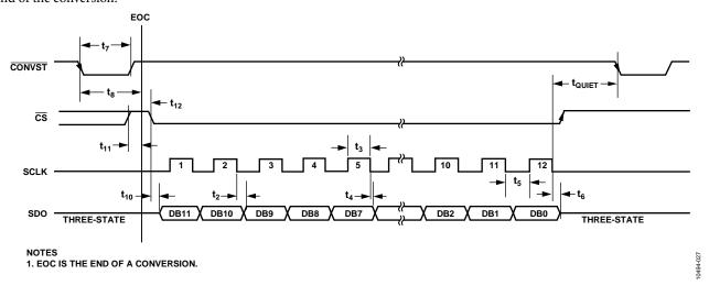
Figure 28. Serial Port Timing Without BUSY Indicator
