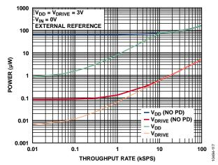
Figure 24. Power Dissipation vs. Throughput Rate (Lower Range)
