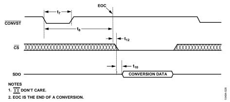
Figure 29. Serial Interface Read Timing—Normal Mode
