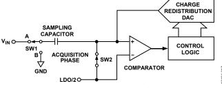
Figure 18. ADC Acquisition Phase
