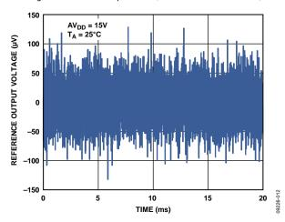
Figure 63. REFOUT Output Noise (100 kHz Bandwidth)
