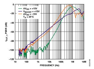
Figure 55. IOUT\_x PSRR vs. Frequency
