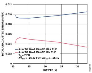
Figure 46. Total Unadjusted Error vs. AV<sub>DD</sub>, External R<sub>SET</sub>
