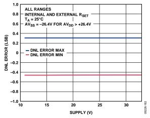
Figure 45. Differential Nonlinearity Error vs. AVDD
