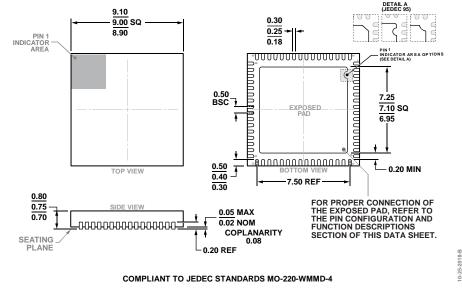
Figure 91. 64-Lead Lead Frame Chip Scale Package [LFCSP] 9 mm × 9 mm Body and 0.75 mm Package Height (CP-64-12) Dimensions shown in millimeters
