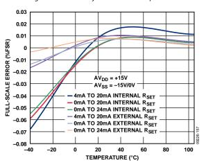
Figure 40. Full Scale Error vs. Temperature
