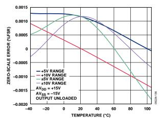
Figure 20. Zero-Scale Error vs. Temperature
