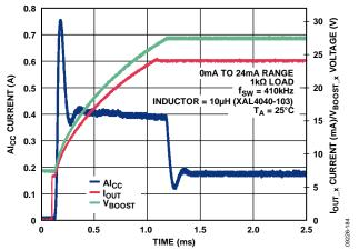
Figure 83. Alcc Current vs. Time for 24 mA Step Through 1  $k\Omega$  Load with Internal Compensation Resistor
