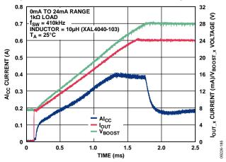
Figure 84. Alcc Current vs. Time for 24 mA Step Through 1 k $\Omega$  Load with External 51 k $\Omega$  Compensation Resistor
