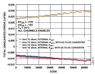
Figure 35. Total Unadjusted Error vs. Code
