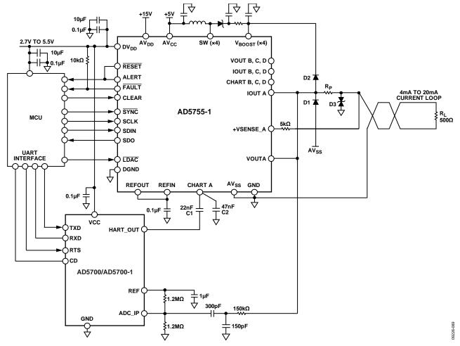
Figure 90. AD5755-1 in HART Configuration
