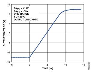
Figure 25. Full-Scale Positive Step
