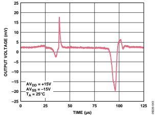
Figure 30.  $V_{OUT_x}$  vs. Time on Power-Up
