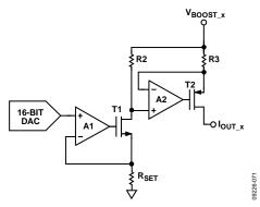
Figure 74. Voltage-to-Current Conversion Circuitry
