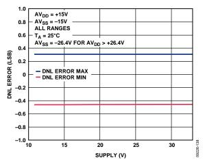
Figure 22. Differential Nonlinearity Error vs. AVDD/|AVSS|
