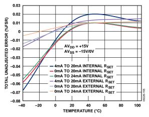
Figure 39. Total Unadjusted Error vs. Temperature
