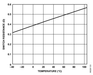
Figure 60. Switch Resistance vs. Temperature
