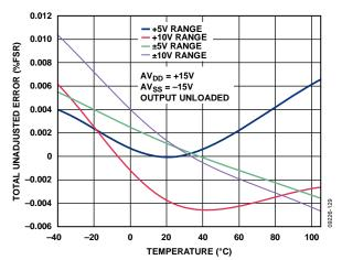
Figure 14. Total Unadjusted Error vs. Temperature
