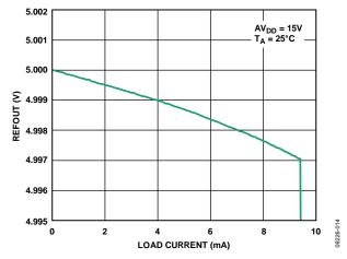
Figure 65. REFOUT vs. Load Current
