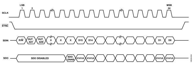
Figure 6. Status Readback During Write
