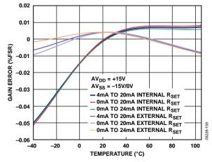
Figure 42. Gain Error vs. Temperature
