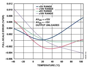
Figure 16. Full-Scale Error vs. Temperature
