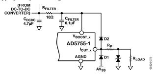
Figure 87. Output Transient Voltage Protection
