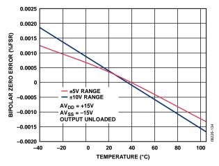
Figure 18. Bipolar Zero Error vs. Temperature
