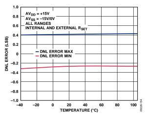
Figure 38. Differential Nonlinearity vs. Temperature
