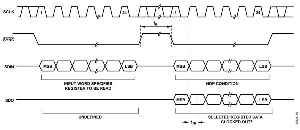
Figure 4. Readback Timing Diagram (Packet Error Checking Disabled)
