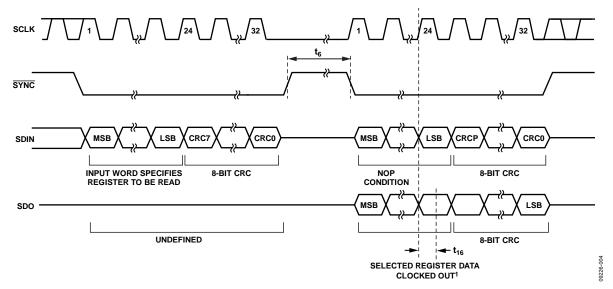
Figure 5. Readback Timing Diagram (Packet Error Checking Enabled)
