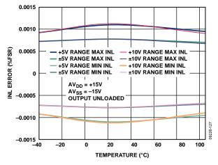
Figure 12. Integral Nonlinearity Error vs. Temperature
