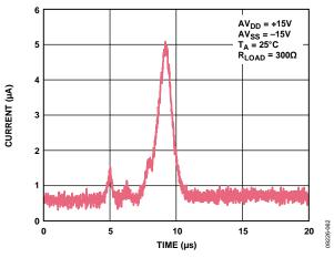
Figure 48. Output Current vs. Time on Power-Up
