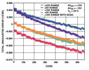
Figure 11. Total Unadjusted Error vs. DAC Code
