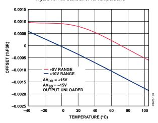
Figure 17. Offset Error vs. Temperature
