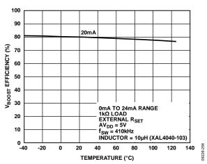
Figure 57. Efficiency at  $V_{BOOST_x}$  vs. Temperature (See Figure 81)
