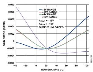
Figure 19. Gain Error vs. Temperature
