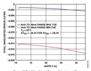
Figure 47. Total Unadjusted Error vs. AV $_{DD}$ , Internal  $R_{SET}$
