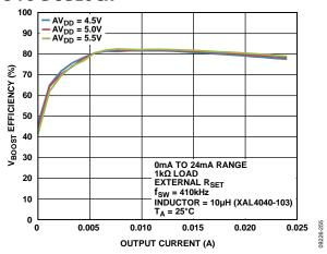
Figure 56. Efficiency at V<sub>BOOST\_x</sub> vs. Output Current (See Figure 81)
