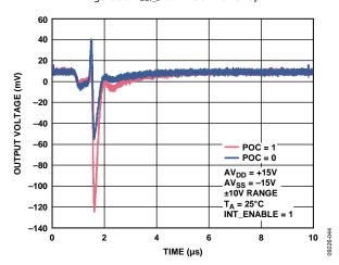
Figure 31. V<sub>OUT\_x</sub> vs. Time on Output Enable
