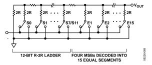
Figure 72. DAC Ladder Structure
