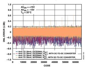
Figure 34. Differential Nonlinearity vs. Code
