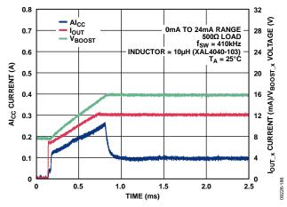
Figure 85. Alcc Current vs. Time for 24 mA Step Through 500  $\Omega$  Load with External 51 k $\Omega$  Compensation Resistor
