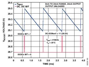
Figure 82. Operation on Reaching V<sub>MAX</sub>
