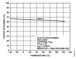
Figure 59. Output Efficiency vs. Temperature (See Figure 81)
