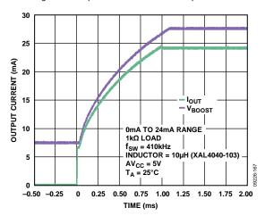
Figure 50. Output Current and V<sub>BOOST\_x</sub> Settling Time with DC-to-DC Converter (See Figure 81)
