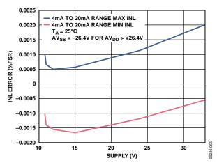
Figure 43. Integral Nonlinearity Error vs. AVDD/|AVSS|, Over Supply, External RSET
