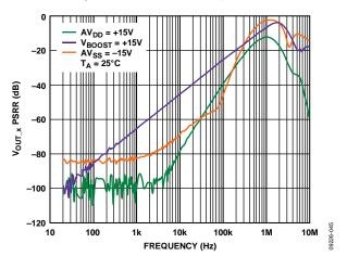
Figure 32. V<sub>OUT\_x</sub> PSRR vs. Frequency
