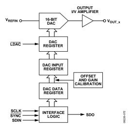
Figure 75. Simplified Serial Interface of Input Loading Circuitry for One DAC Channel
