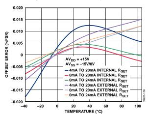
Figure 41. Offset Error vs. Temperature
