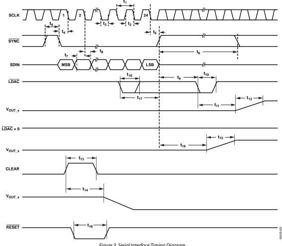
Figure 3. Serial Interface Timing Diagram
