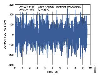
Figure 29. Peak-to-Peak Noise (100 kHz Bandwidth)
