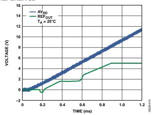
Figure 61. REFOUT Turn-On Transient
