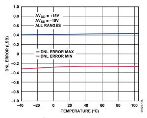
Figure 13. Differential Nonlinearity Error vs. Temperature
