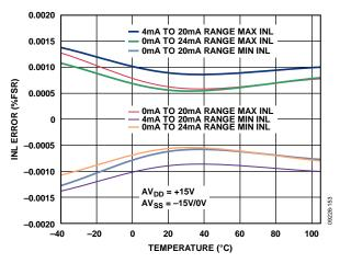
Figure 37. Integral Nonlinearity vs. Temperature, External RSET
