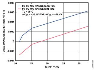
Figure 23. Total Unadjusted Error vs. AVDD/ | AVSS|
