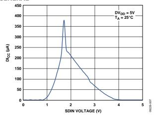
Figure 67. DIcc vs. Logic Input Voltage
