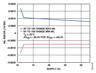
Figure 21. Integral Nonlinearity Error vs. AVDD/|AVSS|
