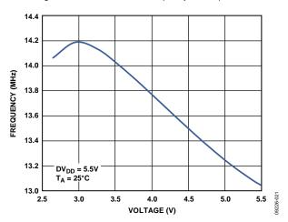
Figure 71. Internal Oscillator Frequency vs. DV<sub>DD</sub> Supply Voltage
