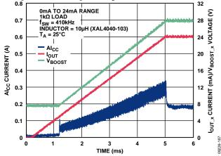
Figure 86. Alcc Current vs. Time for 24 mA Step Through 1 kΩ Load with Slew Rate Control
