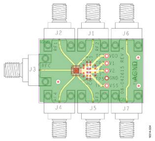
Figure 24. Evaluation Board Component Placement
