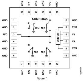
This broadband switch requires dual supply voltages, +3.3 V and -3.3 V, and provides complementary metal-oxide semiconductor (CMOS)/low voltage transistor-transistor logic (LVTTL) logic-compatible control.
