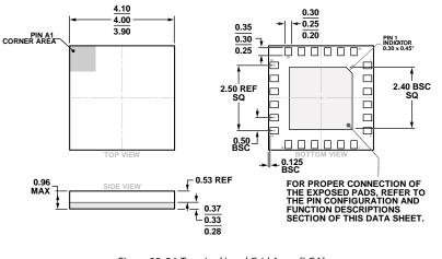
Figure 28. 24-Terminal Land Grid Array [LGA] (CC-24-4) Dimensions shown in millimeters
