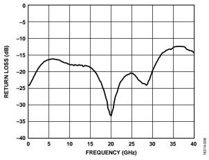
Figure 8. Return Loss vs. Frequency for RFC
