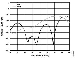
Figure 11. Return Loss vs. Frequency for RF1, RF2, RF3, and RF4
