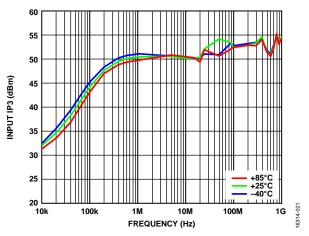
Figure 21. Input IP3 vs. Frequency over Various Temperatures (Low Frequency Detail)
