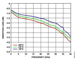
Figure 10. Insertion Loss vs. Frequency over Various Temperatures Between RFC and RF1
