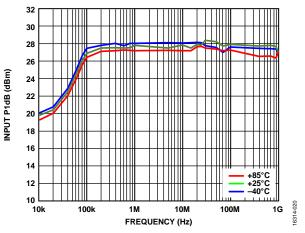
Figure 20. Input 1 dB Power Compression (P1dB) vs. Frequency over Various Temperatures (Low Frequency Detail)
