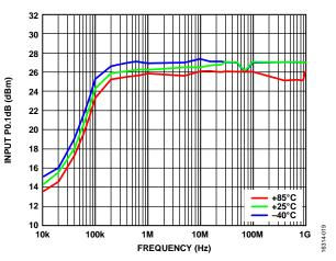
Figure 19. Input 0.1 dB Power Compression (P0.1dB) vs. Frequency over Various Temperatures (Low Frequency Detail)
