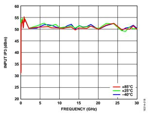
Figure 18. Input IP3 vs. Frequency over Various Temperatures
