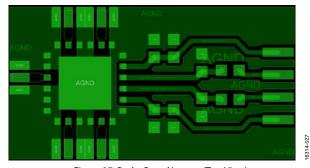
Figure 27. Probe Board Layout (Top View)
