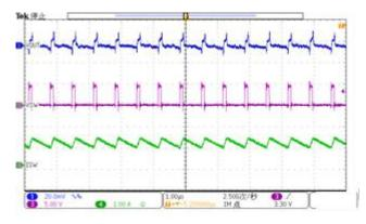
Ripple : VIN=5.0V, VO=0.6V, EN=3.6V IO=1A
