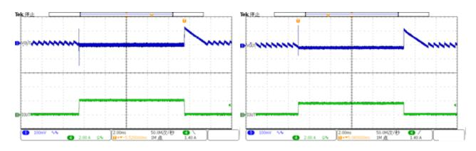
Load Transient Response VIN=5V,VO=1.8V,EN=3.6V,IO=1mA-2A
